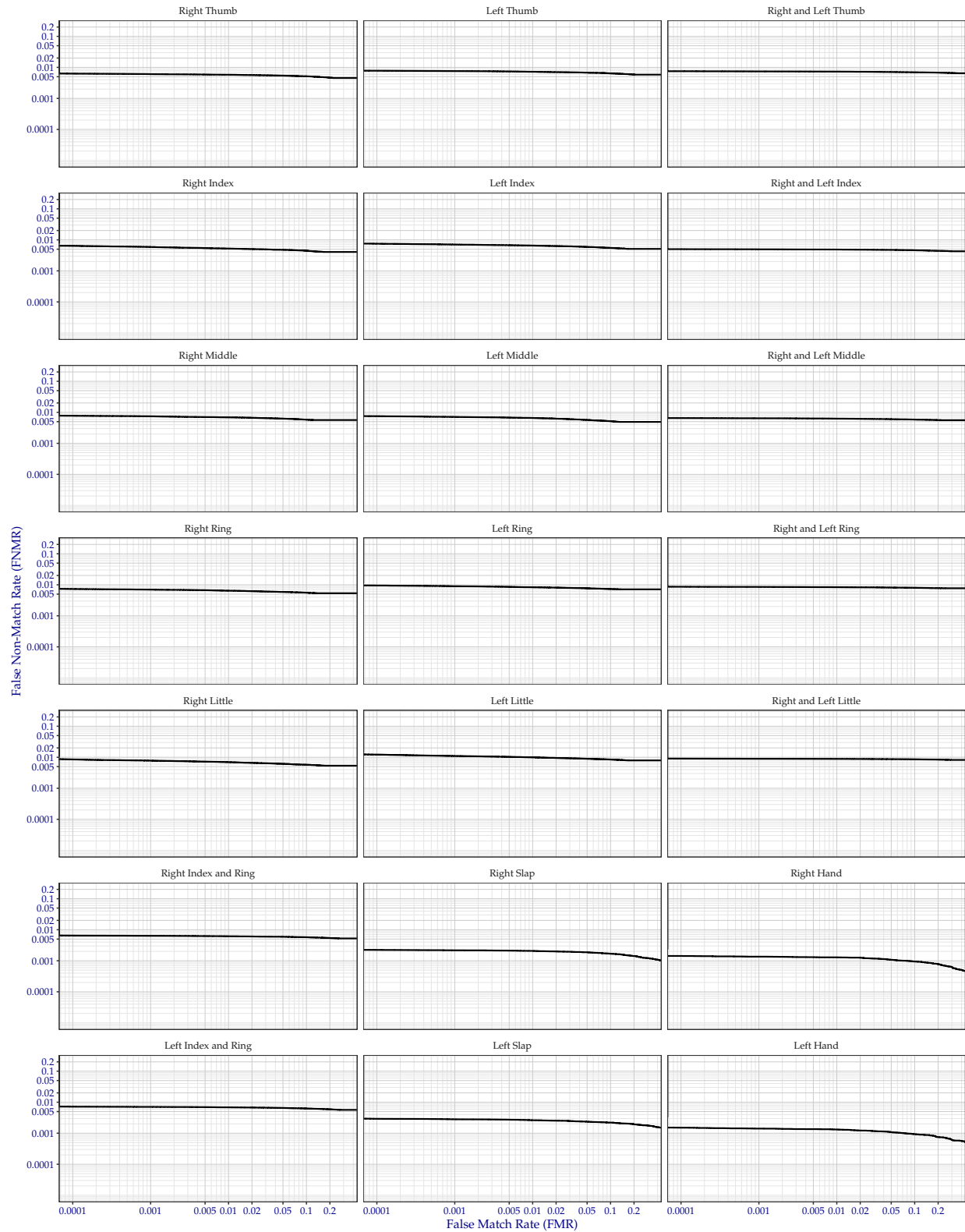
Figure 5: Detection error tradeoff of all comparisons from all fingers in the PFT III AZDPS dataset, separated by finger position. Combined finger positions were generated by sum fusion.
