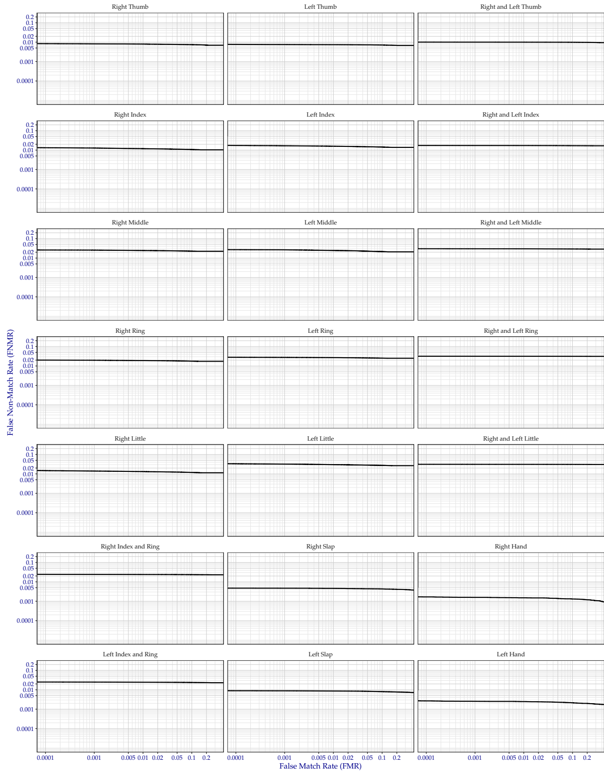
Figure 8: Detection error tradeoff of all comparisons from all fingers in the PFT III LASD dataset, separated by finger position. Combined finger positions were generated by sum fusion.
