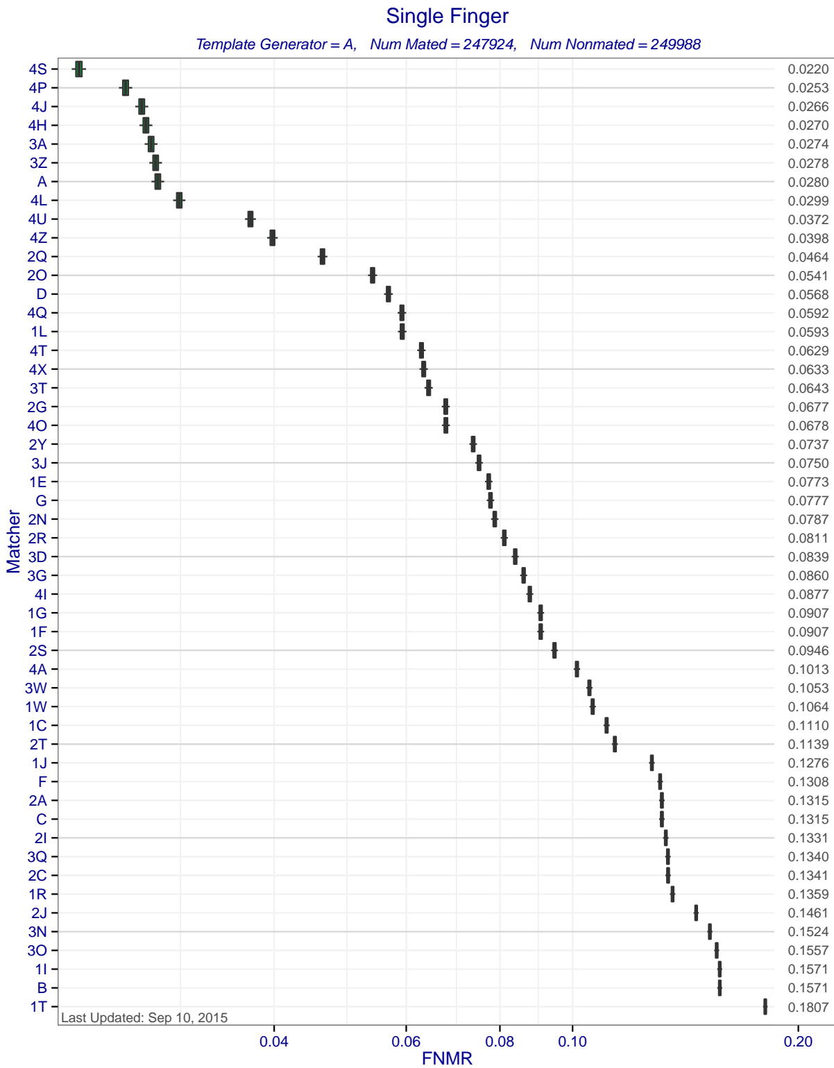
Figure 5: Single Finger FNMRs at FMR=0.0001 when MINEX compliant matchers compare templates created by template generator A. Each box represents uncertainty about the true FNMR. The box edges mark the 50% confidence intervals while the whiskers mark the 90% confidence intervals. The numbers on the right show the actual computed FNMRs.
