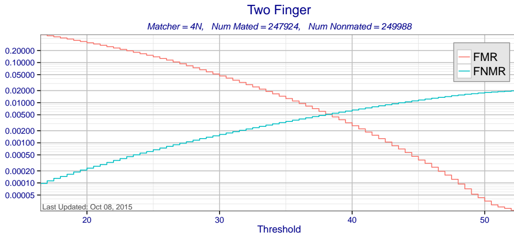
Figure 11: Two finger FMR and FNMR as a function of score threshold for matcher 4N using templates created by all MINEX compliant template generators. Score-level fusion is achieved by averaging scores for the left and right index fingers.
