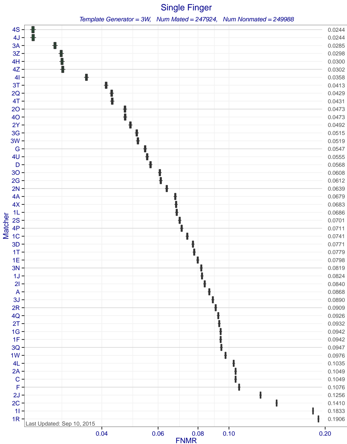
Figure 5: Single Finger FNMRs at FMR=0.0001 when MINEX compliant matchers compare templates created by template generator 3W. Each box represents uncertainty about the true FNMR. The box edges mark the 50% confidence intervals while the whiskers mark the 90% confidence intervals. The numbers on the right show the actual computed FNMRs.
