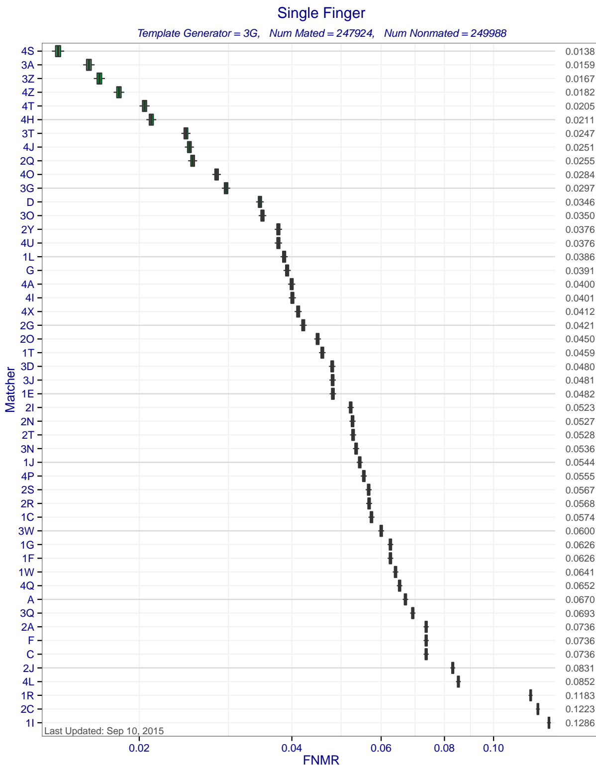
Figure 5: Single Finger FNMRs at FMR=0.0001 when MINEX compliant matchers compare templates created by template generator 3G. Each box represents uncertainty about the true FNMR. The box edges mark the 50% confidence intervals while the whiskers mark the 90% confidence intervals. The numbers on the right show the actual computed FNMRs.
