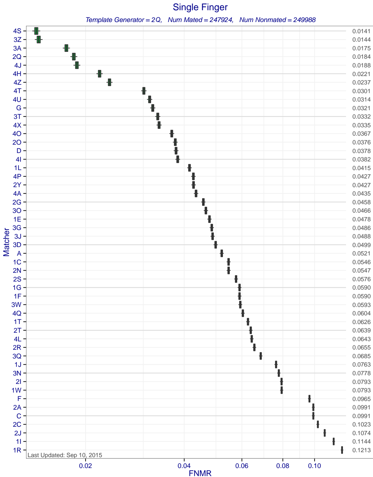
Figure 5: Single Finger FNMRs at FMR=0.0001 when MINEX compliant matchers compare templates created by template generator 2Q. Each box represents uncertainty about the true FNMR. The box edges mark the 50% confidence intervals while the whiskers mark the 90% confidence intervals. The numbers on the right show the actual computed FNMRs.
