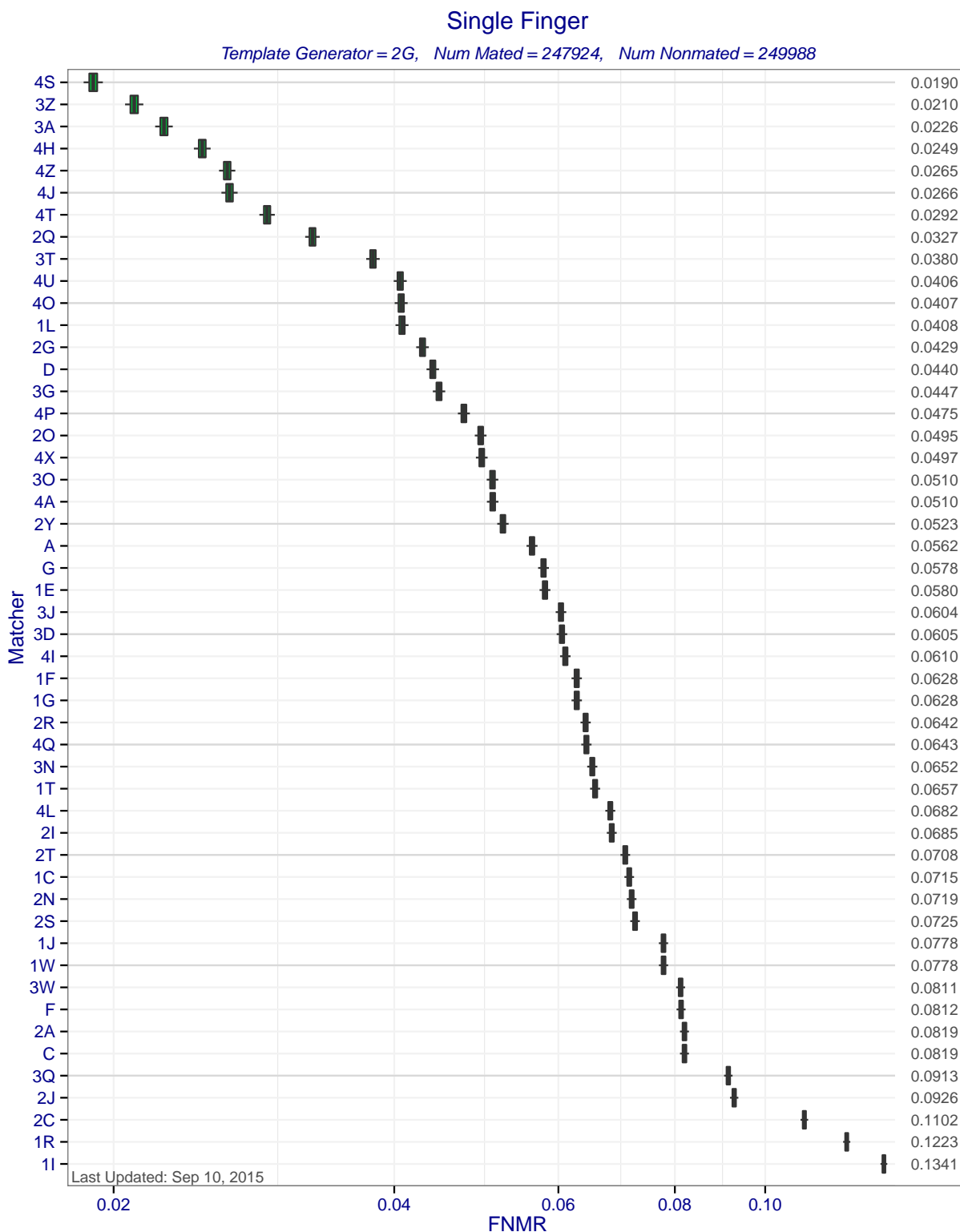
Figure 5: Single Finger FNMRs at FMR=0.0001 when MINEX compliant matchers compare templates created by template generator 2G. Each box represents uncertainty about the true FNMR. The box edges mark the 50% confidence intervals while the whiskers mark the 90% confidence intervals. The numbers on the right show the actual computed FNMRs.
