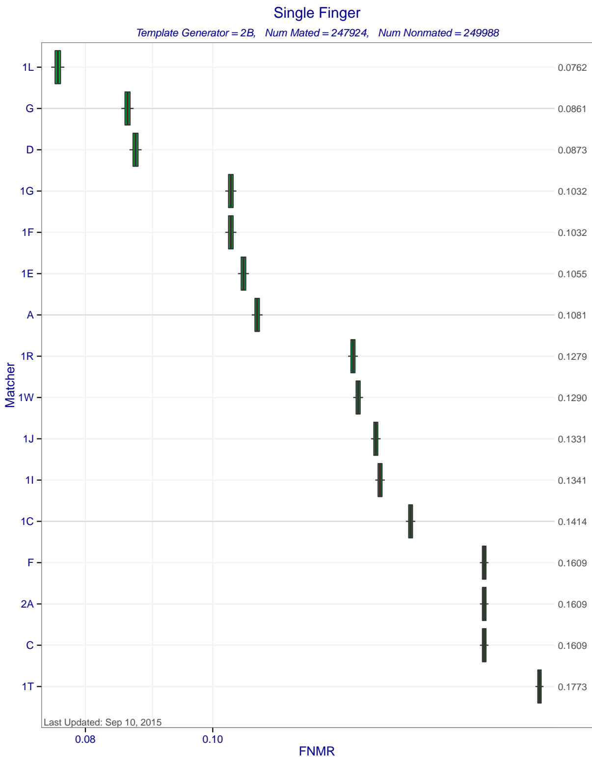
Figure 5: Single Finger FNMRs at FMR=0.0001 when MINEX compliant matchers compare templates created by template generator 2B. Each box represents uncertainty about the true FNMR. The box edges mark the 50% confidence intervals while the whiskers mark the 90% confidence intervals. The numbers on the right show the actual computed FNMRs.
