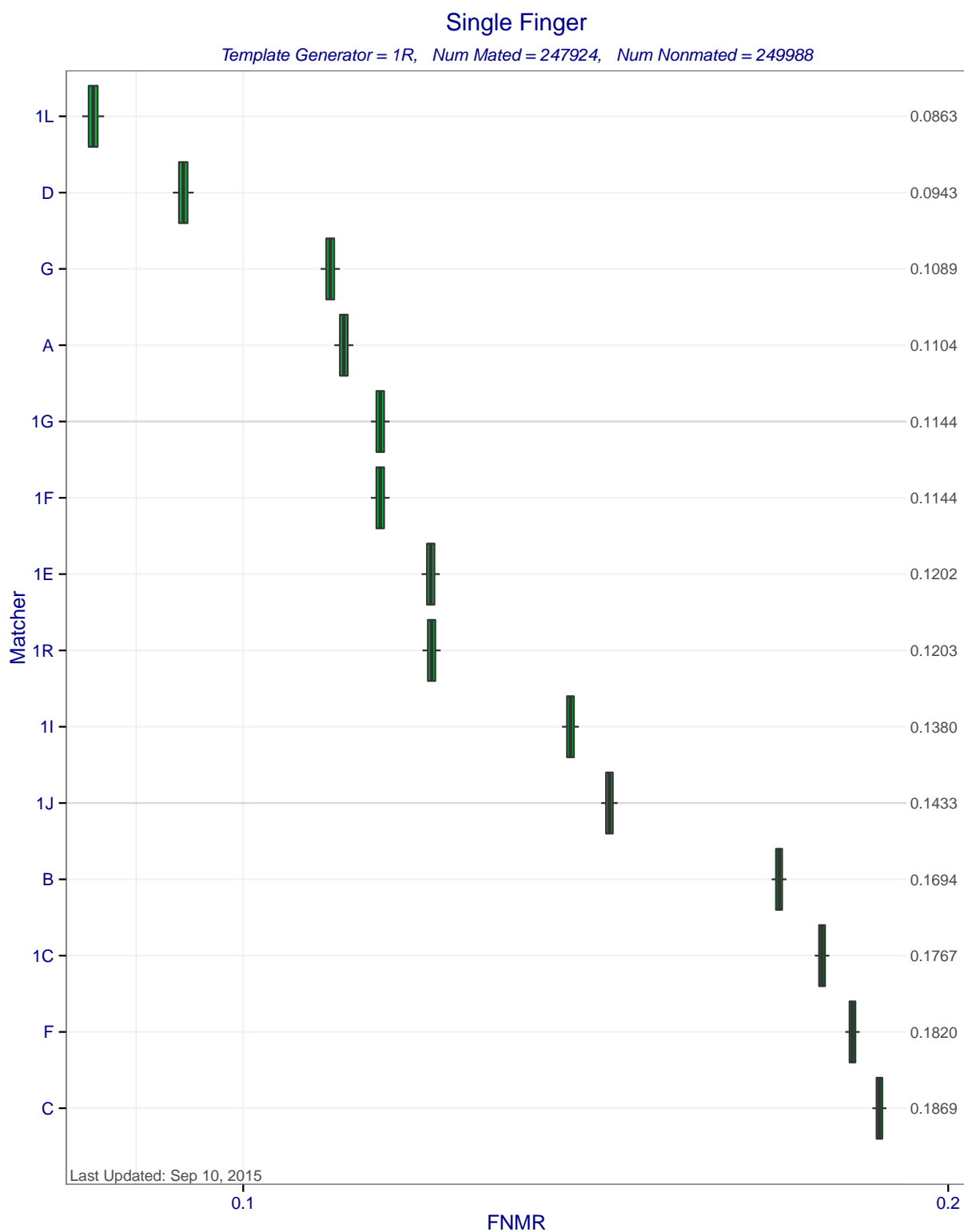
Figure 5: Single Finger FNMRs at FMR=0.0001 when MINEX compliant matchers compare templates created by template generator 1R. Each box represents uncertainty about the true FNMR. The box edges mark the 50% confidence intervals while the whiskers mark the 90% confidence intervals. The numbers on the right show the actual computed FNMRs.
