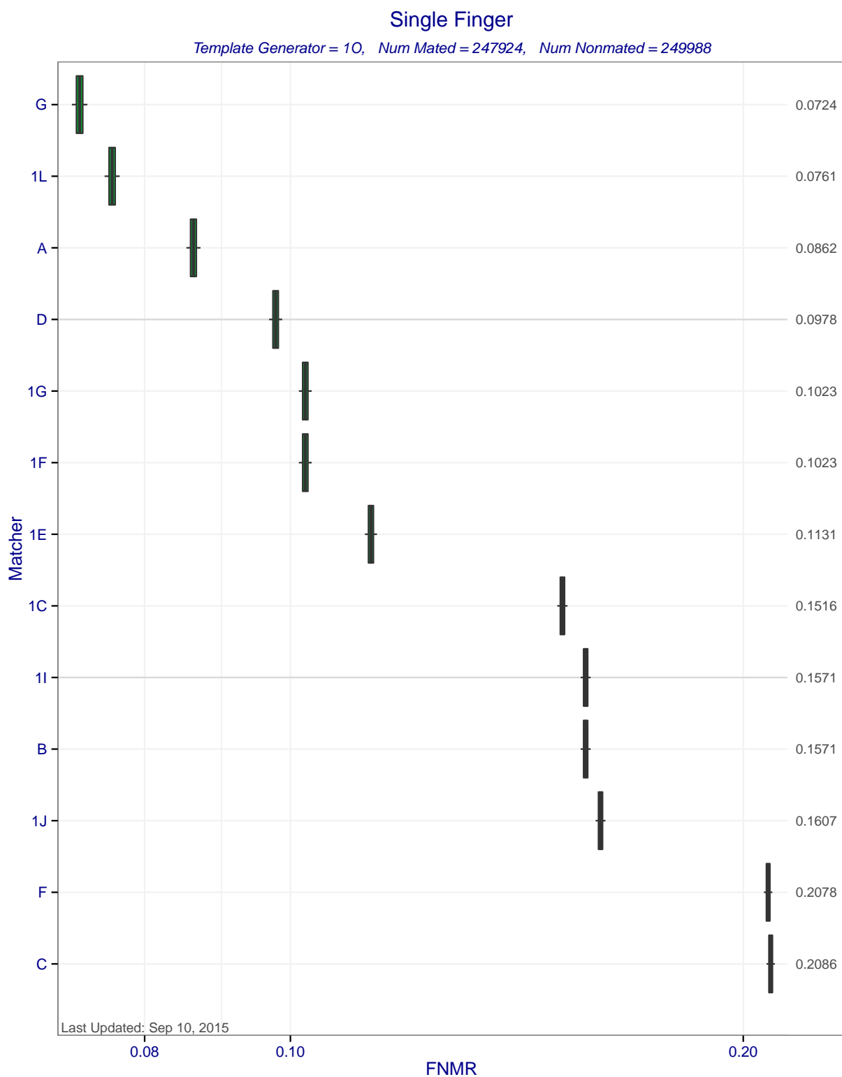
Figure 5: Single Finger FNMRs at FMR=0.0001 when MINEX compliant matchers compare templates created by template generator 10. Each box represents uncertainty about the true FNMR. The box edges mark the 50% confidence intervals while the whiskers mark the 90% confidence intervals. The numbers on the right show the actual computed FNMRs.
