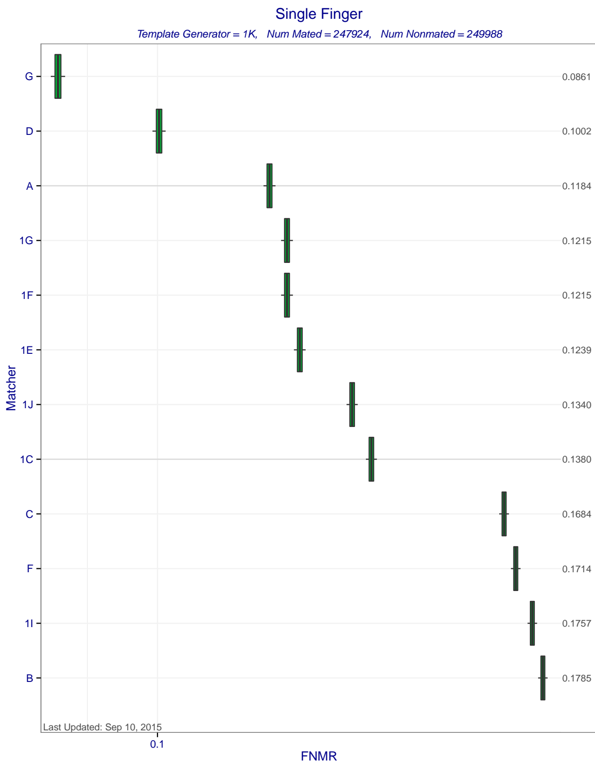
Figure 5: Single Finger FNMRs at FMR=0.0001 when MINEX compliant matchers compare templates created by template generator 1K. Each box represents uncertainty about the true FNMR. The box edges mark the 50% confidence intervals while the whiskers mark the 90% confidence intervals. The numbers on the right show the actual computed FNMRs.
