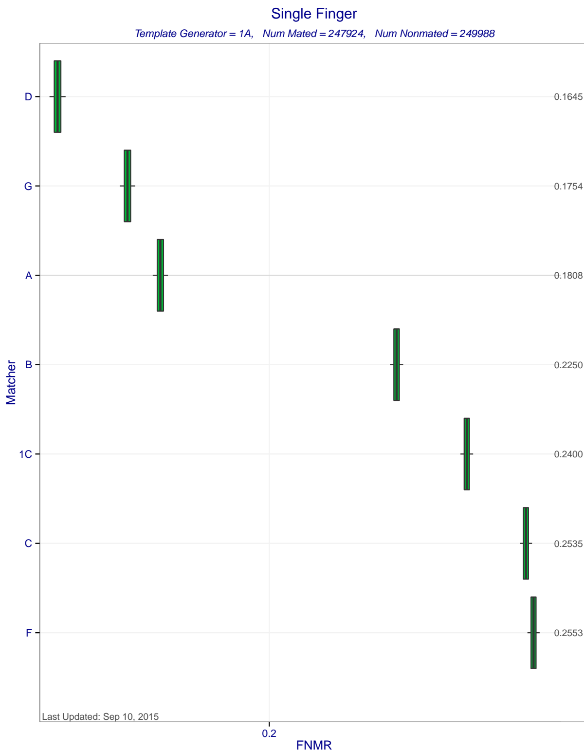
Figure 5: Single Finger FNMRs at FMR=0.0001 when MINEX compliant matchers compare templates created by template generator 1A. Each box represents uncertainty about the true FNMR. The box edges mark the 50% confidence intervals while the whiskers mark the 90% confidence intervals. The numbers on the right show the actual computed FNMRs.
