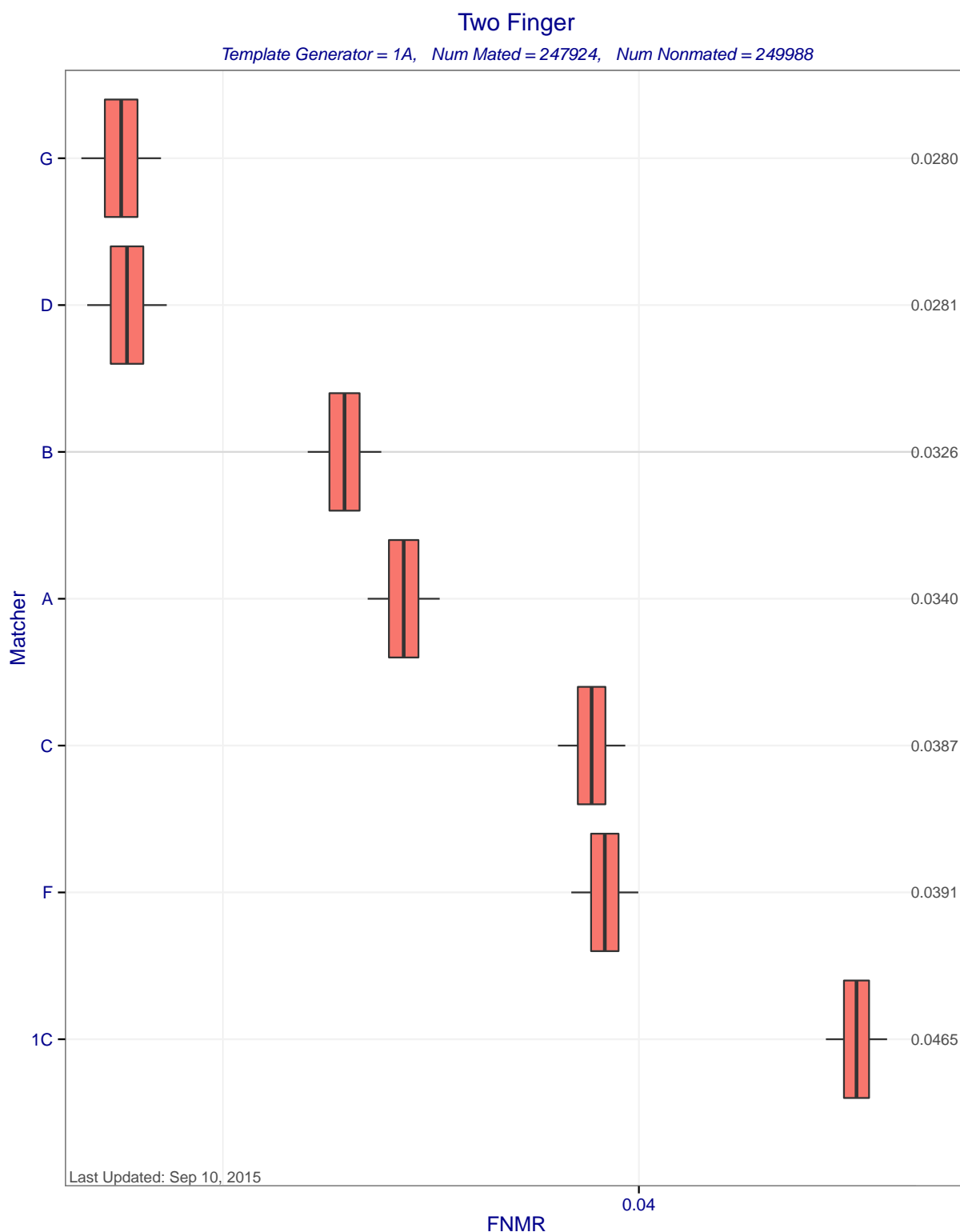
Figure 7: Two Finger FNMR at FMR=0.01 when different matchers compare templates created by template generator 1A. Each box represents uncertainty about the true FNMR. The box edges mark the 50% confidence intervals while the whiskers mark the 90% confidence intervals. The numbers on the right show the actual computed FNMRs. Score-level fusion is achieved by averaging the scores for left and right index fingers.
