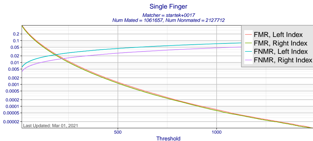
Figure 11: Single finger FMR and FNMR as a function of score threshold for matcher startek+0017 using templates created by all MINEX III compliant template generators. Separate curves are presented for left and right index fingers.
