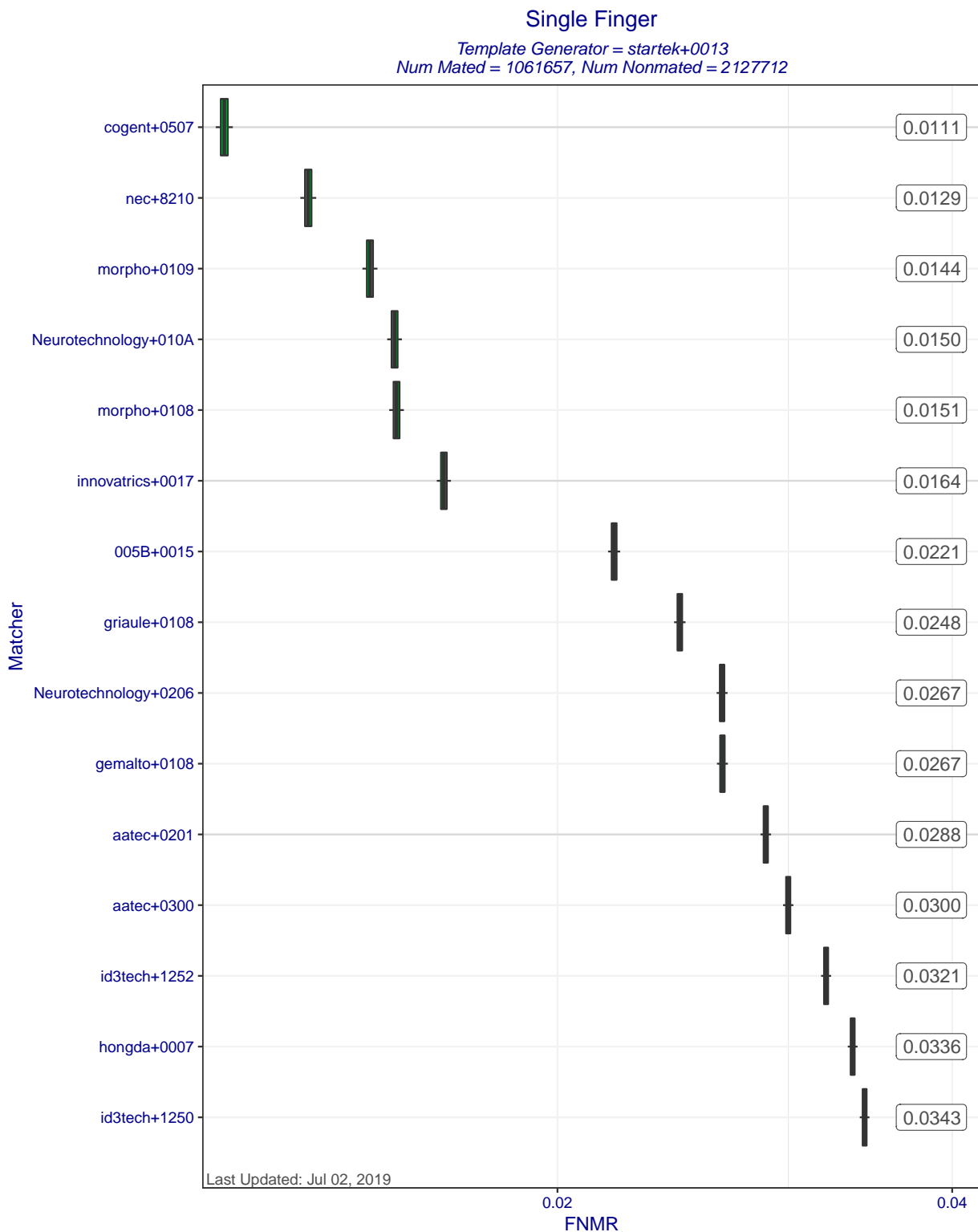
Figure 5: Single Finger FNMRs at FMR=0.0001 when MINEX III compliant matchers compare templates created by template generator startek+0013. Each box represents uncertainty about the true FNMR. The box edges mark the 50% confidence intervals while the whiskers mark the 90% confidence intervals. The numbers on the right show the actual computed FNMRs.
