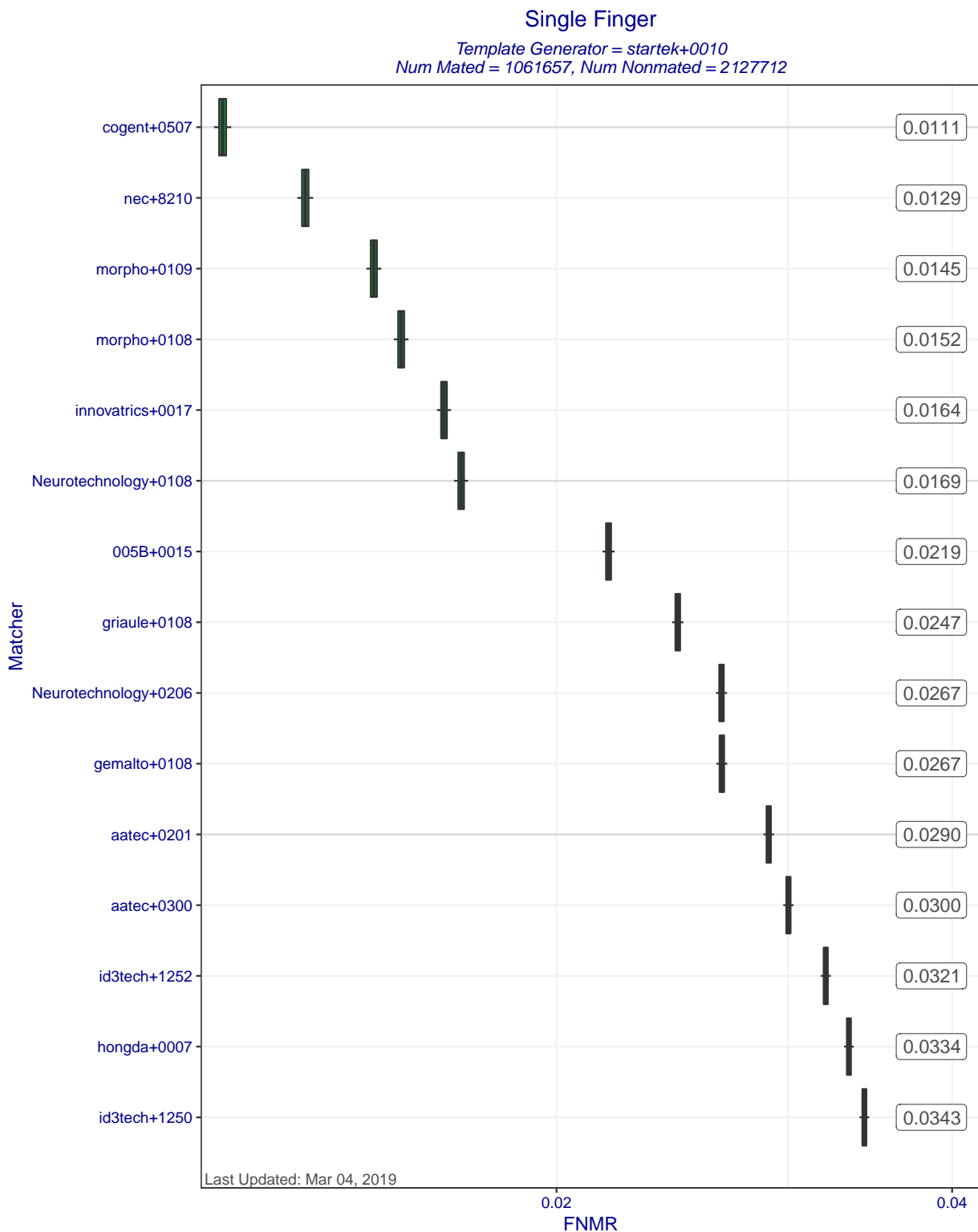
Figure 5: Single Finger FNMRs at FMR=0.0001 when MINEX III compliant matchers compare templates created by template generator startek+0010. Each box represents uncertainty about the true FNMR. The box edges mark the 50% confidence intervals while the whiskers mark the 90% confidence intervals. The numbers on the right show the actual computed FNMRs.
