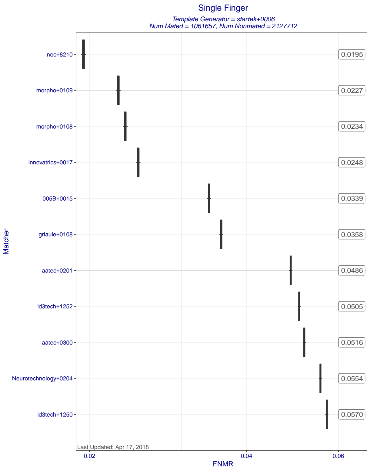
Figure 5: Single Finger FNMRs at FMR=0.0001 when MINEX III compliant matchers compare templates created by template generator startek+0006. Each box represents uncertainty about the true FNMR. The box edges mark the 50% confidence intervals while the whiskers mark the 90% confidence intervals. The numbers on the right show the actual computed FNMRs.
