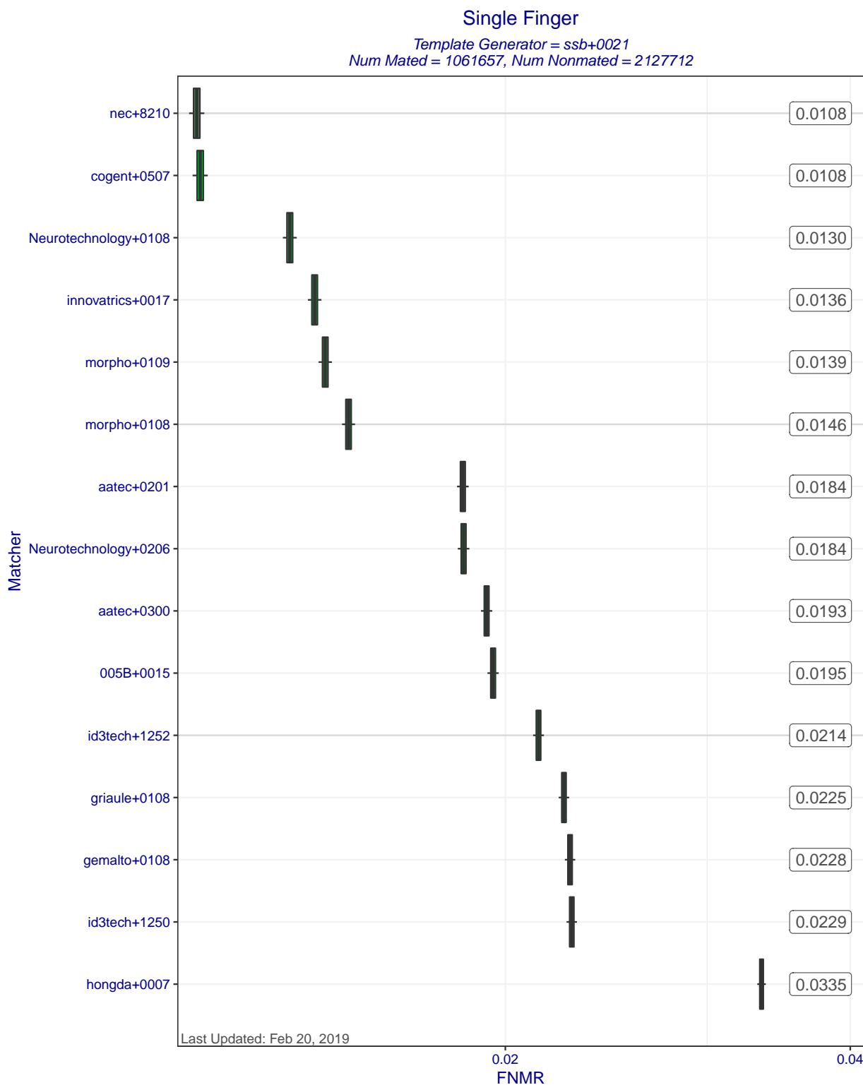
Figure 5: Single Finger FNMRs at FMR=0.0001 when MINEX III compliant matchers compare templates created by template generator ssb+0021. Each box represents uncertainty about the true FNMR. The box edges mark the 50% confidence intervals while the whiskers mark the 90% confidence intervals. The numbers on the right show the actual computed FNMRs.
