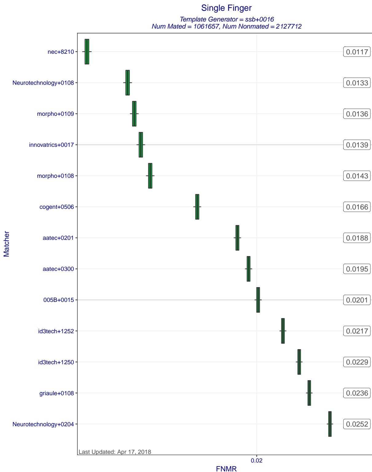
Figure 5: Single Finger FNMRs at FMR=0.0001 when MINEX III compliant matchers compare templates created by template generator ssb+0016. Each box represents uncertainty about the true FNMR. The box edges mark the 50% confidence intervals while the whiskers mark the 90% confidence intervals. The numbers on the right show the actual computed FNMRs.
