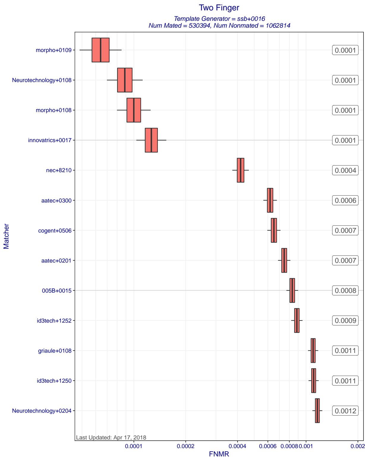
Figure 7: Two Finger FNMR at FMR=0.01 when different matchers compare templates created by template generator ssb+0016 . Each box represents uncertainty about the true FNMR. The box edges mark the 50% confidence intervals while the whiskers mark the 90% confidence intervals. The numbers on the right show the actual computed FNMRs. Score-level fusion is achieved by averaging the scores for left and right index fingers.
