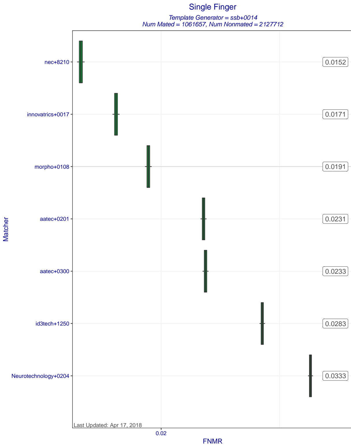
Figure 5: Single Finger FNMRs at FMR=0.0001 when MINEX III compliant matchers compare templates created by template generator ssb+0014. Each box represents uncertainty about the true FNMR. The box edges mark the 50% confidence intervals while the whiskers mark the 90% confidence intervals. The numbers on the right show the actual computed FNMRs.
