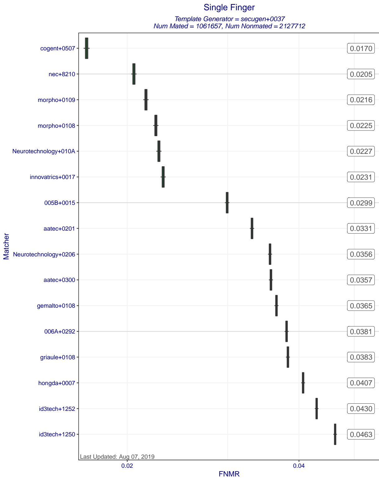
Figure 5: Single Finger FNMRs at FMR=0.0001 when MINEX III compliant matchers compare templates created by template generator secugen+0037. Each box represents uncertainty about the true FNMR. The box edges mark the 50% confidence intervals while the whiskers mark the 90% confidence intervals. The numbers on the right show the actual computed FNMRs.
