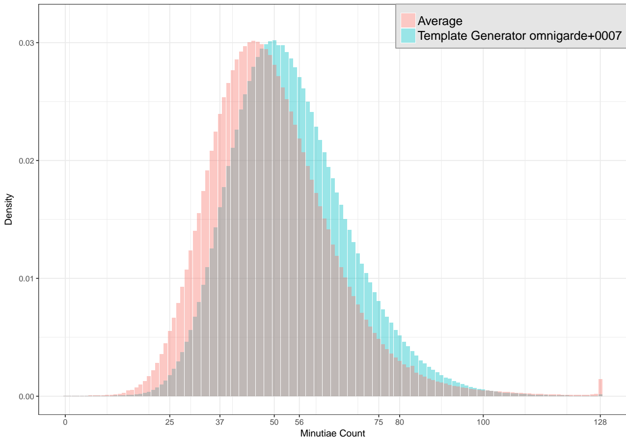
Figure 3: Probability distribution of the number of minutia the template generator found in the samples. The average probability distribution shows the combined distribution of minutia counts across all compliant template generators submitted for MINEX III (i.e., excluding Ongoing MINEX template generators).
