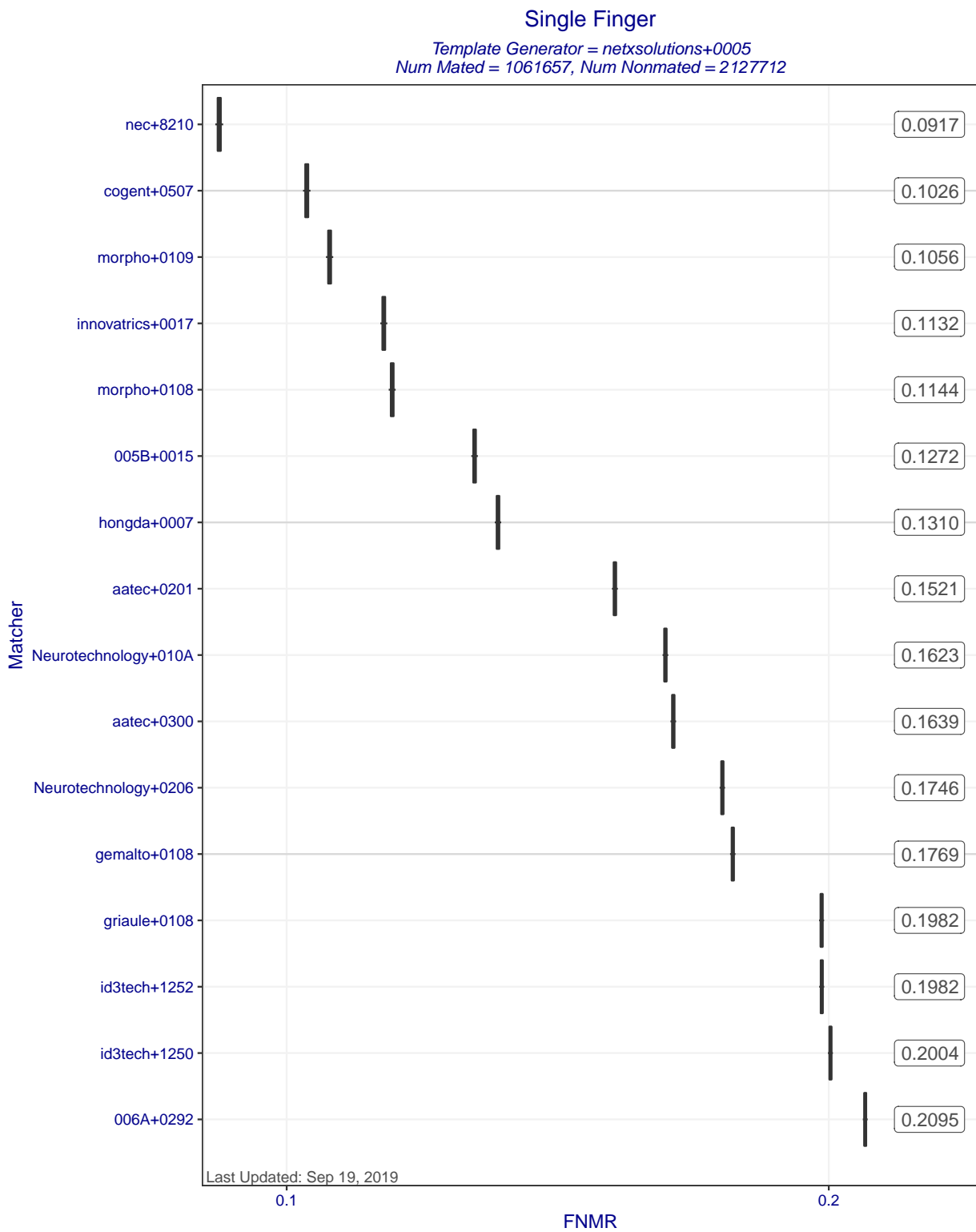
Figure 5: Single Finger FNMRs at FMR=0.0001 when MINEX III compliant matchers compare templates created by template generator netxsolutions+0005. Each box represents uncertainty about the true FNMR. The box edges mark the 50% confidence intervals while the whiskers mark the 90% confidence intervals. The numbers on the right show the actual computed FNMRs.
