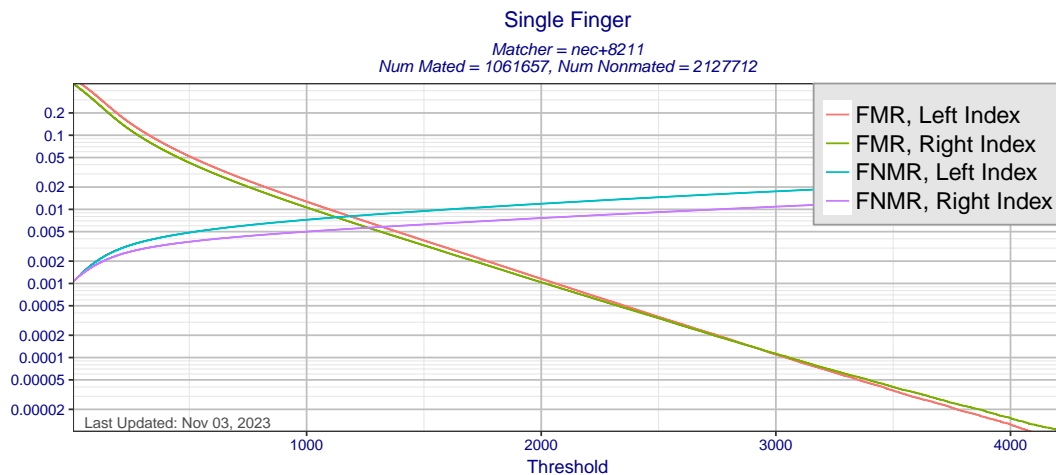
Figure 11: Single finger FMR and FNMR as a function of score threshold for matcher nec+8211 using templates created by all MINEX III compliant template generators. Separate curves are presented for left and right index fingers.
