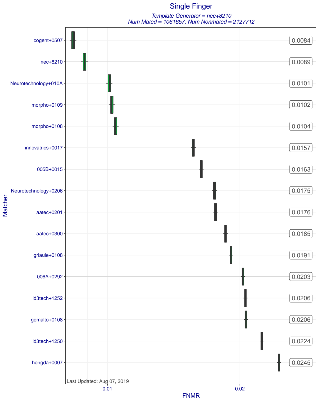
Figure 5: Single Finger FNMRs at FMR=0.0001 when MINEX III compliant matchers compare templates created by template generator nec+8210. Each box represents uncertainty about the true FNMR. The box edges mark the 50% confidence intervals while the whiskers mark the 90% confidence intervals. The numbers on the right show the actual computed FNMRs.
