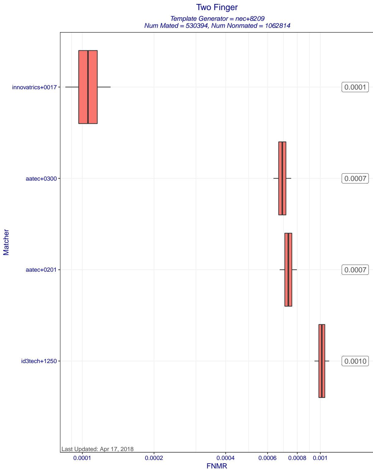
Figure 7: Two Finger FNMR at FMR=0.01 when different matchers compare templates created by template generator nec+8209. Each box represents uncertainty about the true FNMR. The box edges mark the 50% confidence intervals while the whiskers mark the 90% confidence intervals. The numbers on the right show the actual computed FNMRs. Score-level fusion is achieved by averaging the scores for left and right index fingers.
