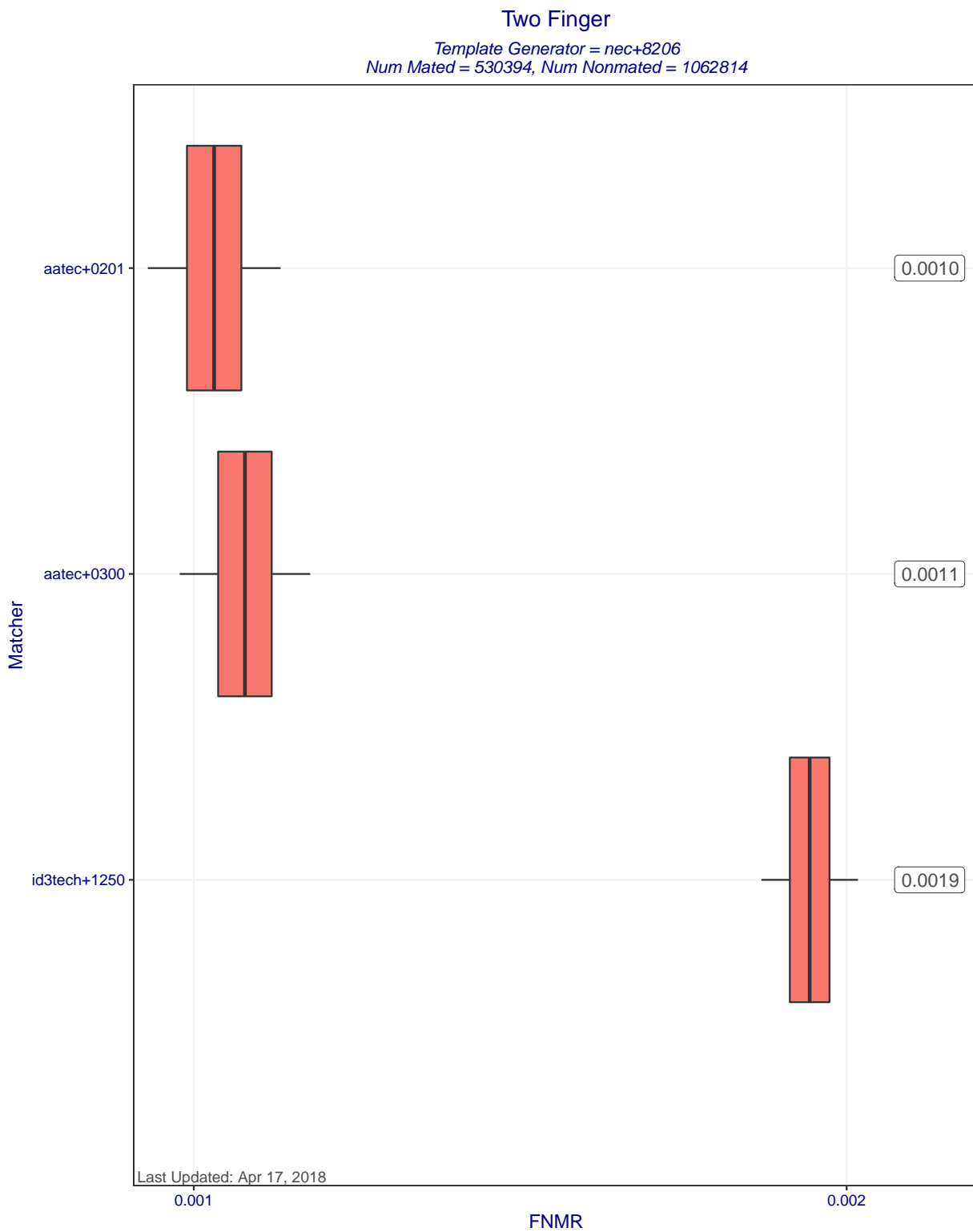
Figure 7: Two Finger FNMR at FMR=0.01 when different matchers compare templates created by template generator nec+8206. Each box represents uncertainty about the true FNMR. The box edges mark the 50% confidence intervals while the whiskers mark the 90% confidence intervals. The numbers on the right show the actual computed FNMRs. Score-level fusion is achieved by averaging the scores for left and right index fingers.
