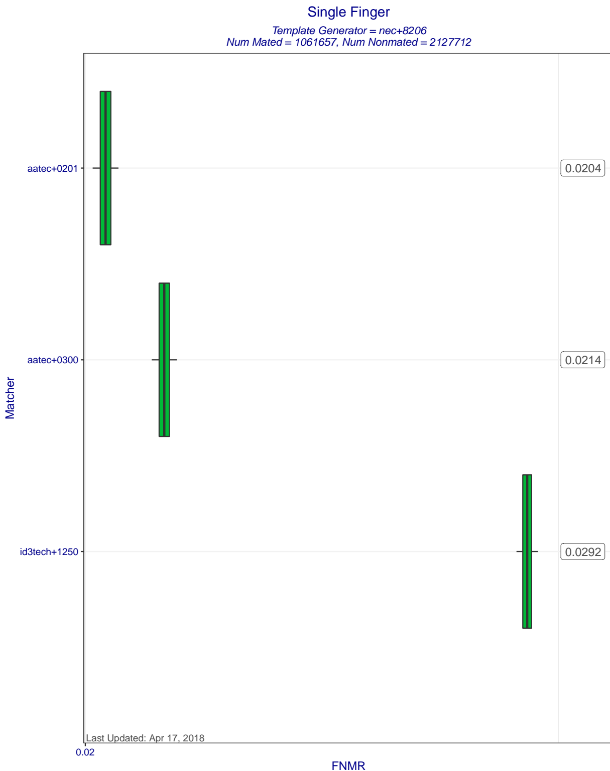
Figure 5: Single Finger FNMRs at FMR=0.0001 when MINEX III compliant matchers compare templates created by template generator nec+8206. Each box represents uncertainty about the true FNMR. The box edges mark the 50% confidence intervals while the whiskers mark the 90% confidence intervals. The numbers on the right show the actual computed FNMRs.
