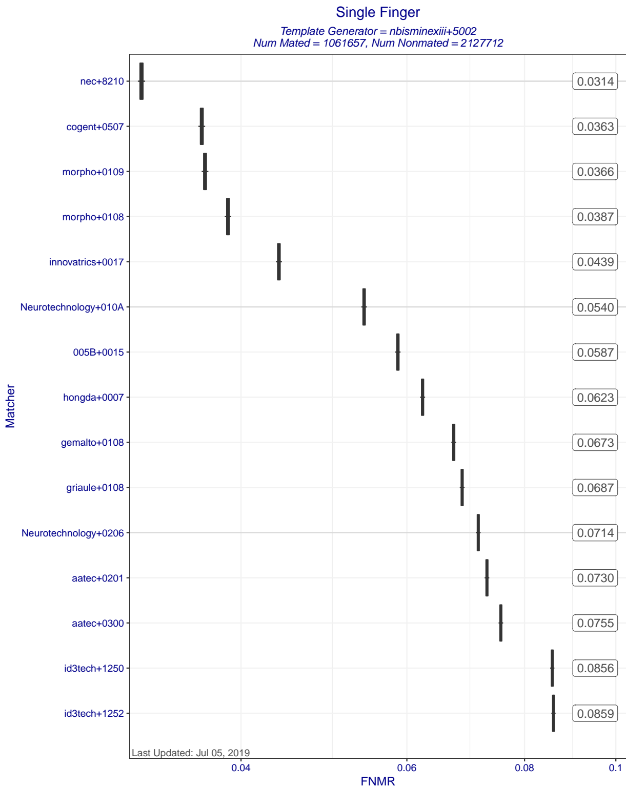
Figure 5: Single Finger FNMRs at FMR=0.0001 when MINEX III compliant matchers compare templates created by template generator nbisminexiii+5002. Each box represents uncertainty about the true FNMR. The box edges mark the 50% confidence intervals while the whiskers mark the 90% confidence intervals. The numbers on the right show the actual computed FNMRs.
