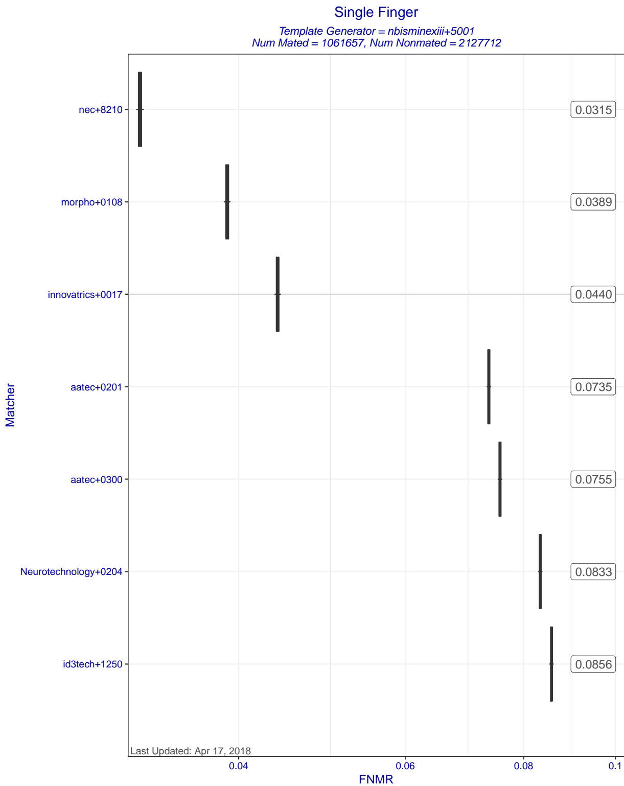
Figure 5: Single Finger FNMRs at FMR=0.0001 when MINEX III compliant matchers compare templates created by template generator nbisminexiii+5001. Each box represents uncertainty about the true FNMR. The box edges mark the 50% confidence intervals while the whiskers mark the 90% confidence intervals. The numbers on the right show the actual computed FNMRs.
