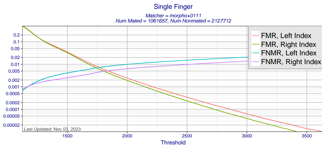
Figure 11: Single finger FMR and FNMR as a function of score threshold for matcher morpho+0111 using templates created by all MINEX III compliant template generators. Separate curves are presented for left and right index fingers.
