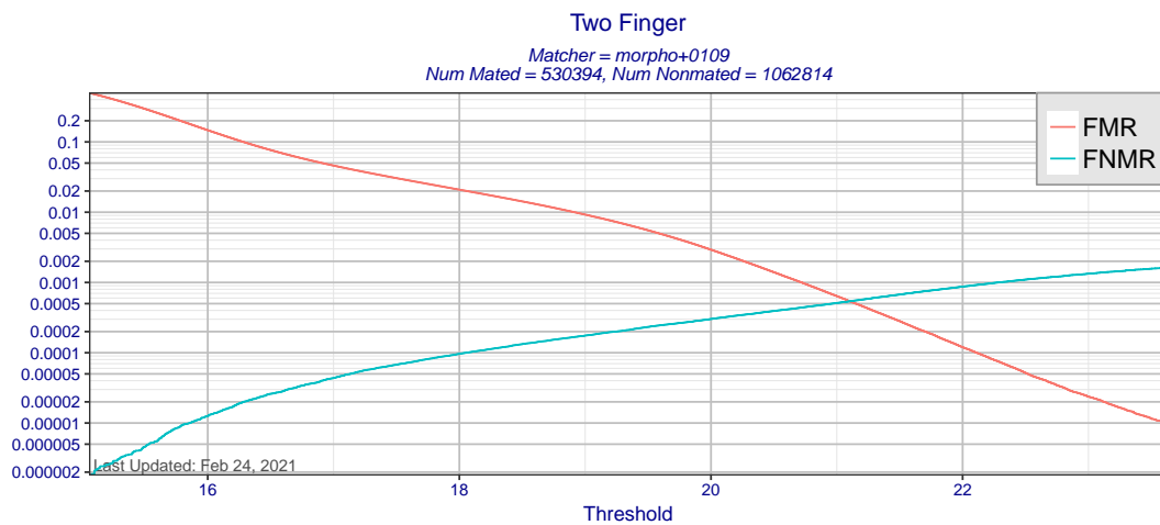
Figure 12: Two finger FMR and FNMR as a function of score threshold for matcher morpho+0109 using templates created by all MINEX III compliant template generators. Score-level fusion is achieved by averaging scores for the left and right index fingers.
