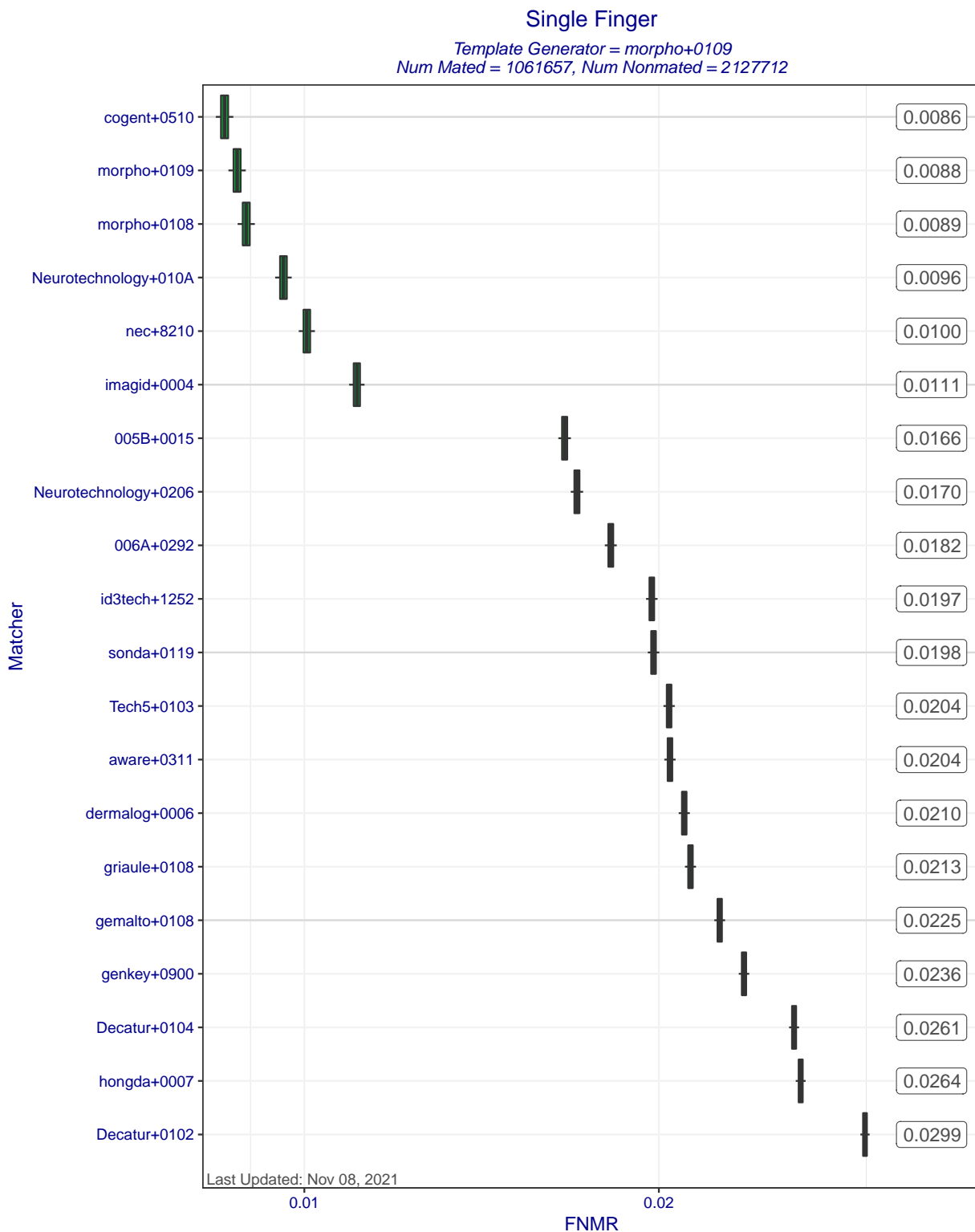
Figure 5: Single Finger FNMRs at FMR=0.0001 when MINEX III compliant matchers compare templates created by template generator morpho+0109. Each box represents uncertainty about the true FNMR. The box edges mark the 50% confidence intervals while the whiskers mark the 90% confidence intervals. The numbers on the right show the actual computed FNMRs.
