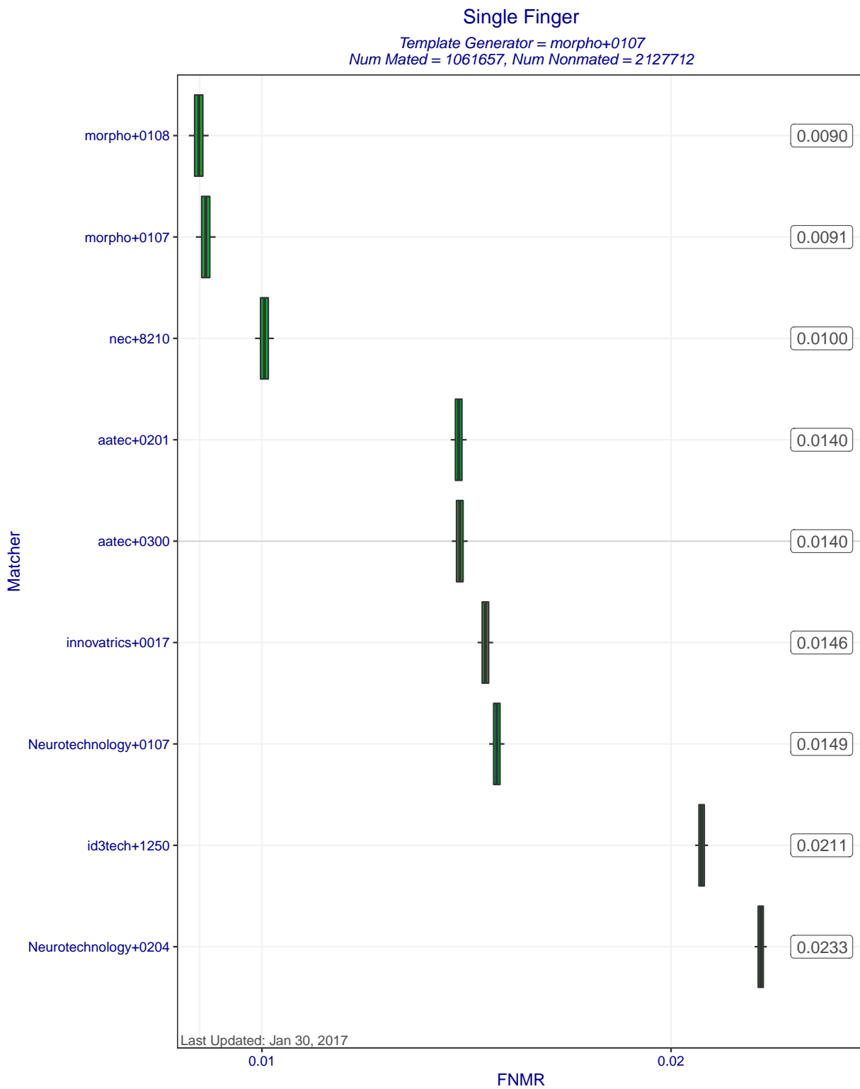
Figure 5: Single Finger FNMRs at FMR=0.0001 when MINEX III compliant matchers compare templates created by template generator morpho+0107. Each box represents uncertainty about the true FNMR. The box edges mark the 50% confidence intervals while the whiskers mark the 90% confidence intervals. The numbers on the right show the actual computed FNMRs.
