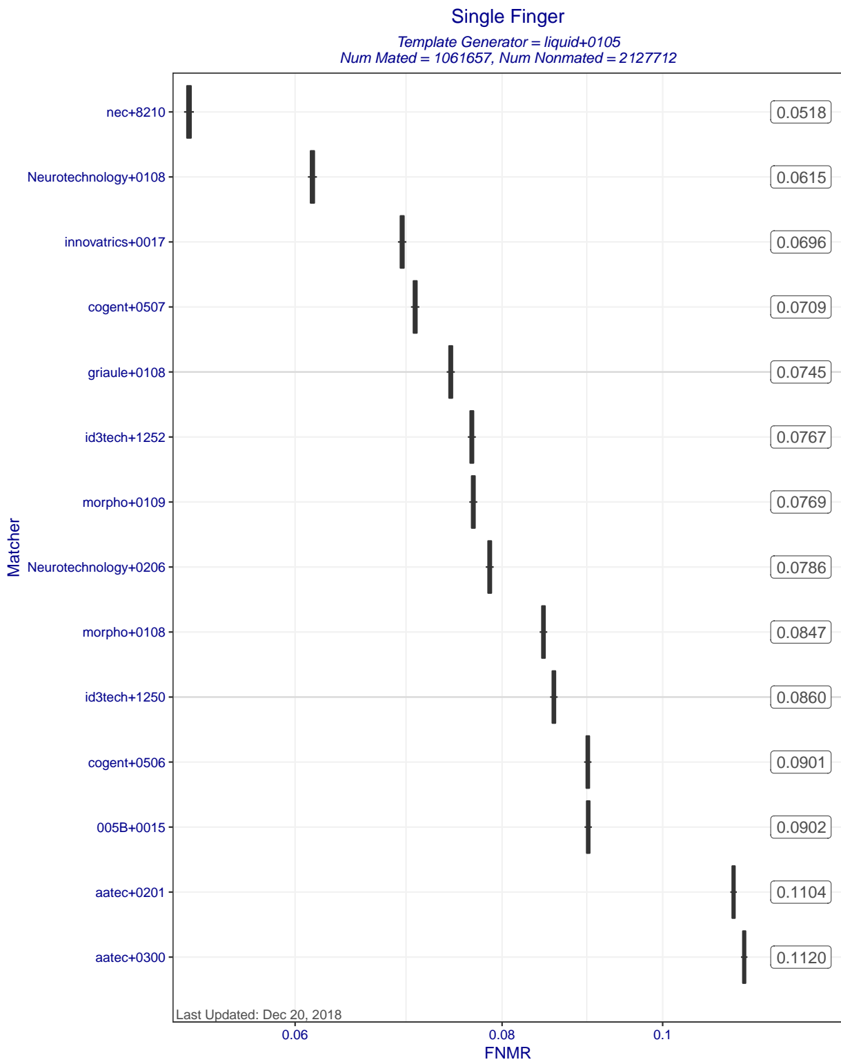
Figure 5: Single Finger FNMRs at FMR=0.0001 when MINEX III compliant matchers compare templates created by template generator liquid+0105. Each box represents uncertainty about the true FNMR. The box edges mark the 50% confidence intervals while the whiskers mark the 90% confidence intervals. The numbers on the right show the actual computed FNMRs.
