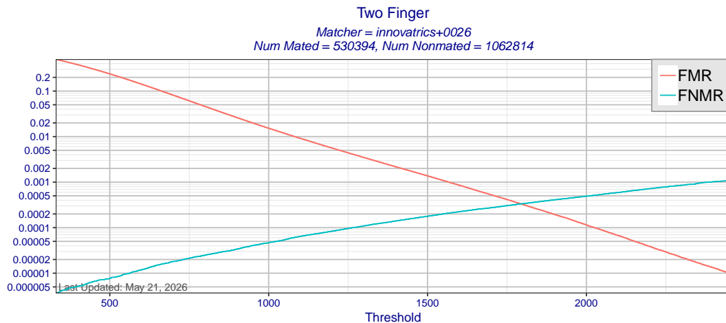
Figure 12: Two finger FMR and FNMR as a function of score threshold for matcher innovatrics+0026 using templates created by all MINEX III compliant template generators. Score-level fusion is achieved by averaging scores for the left and right index fingers.
