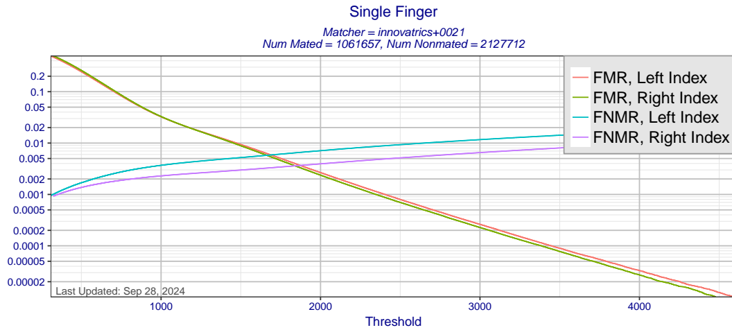
Figure 11: Single finger FMR and FNMR as a function of score threshold for matcher innovatrics+0021 using templates created by all MINEX III compliant template generators. Separate curves are presented for left and right index fingers.
