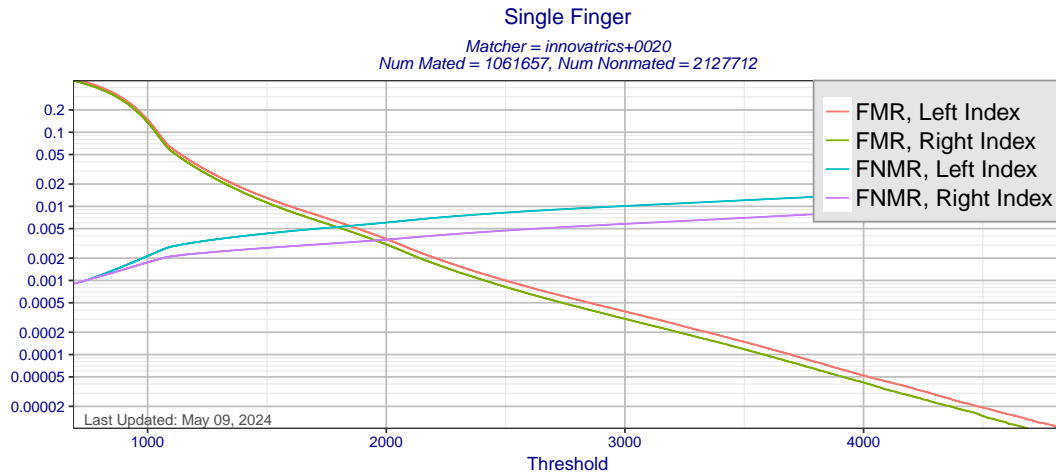
Figure 11: Single finger FMR and FNMR as a function of score threshold for matcher innovatrics+0020 using templates created by all MINEX III compliant template generators. Separate curves are presented for left and right index fingers.
