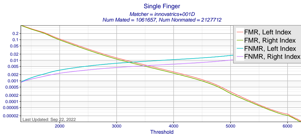
Figure 11: Single finger FMR and FNMR as a function of score threshold for matcher innovatrics+001D using templates created by all MINEX III compliant template generators. Separate curves are presented for left and right index fingers.
