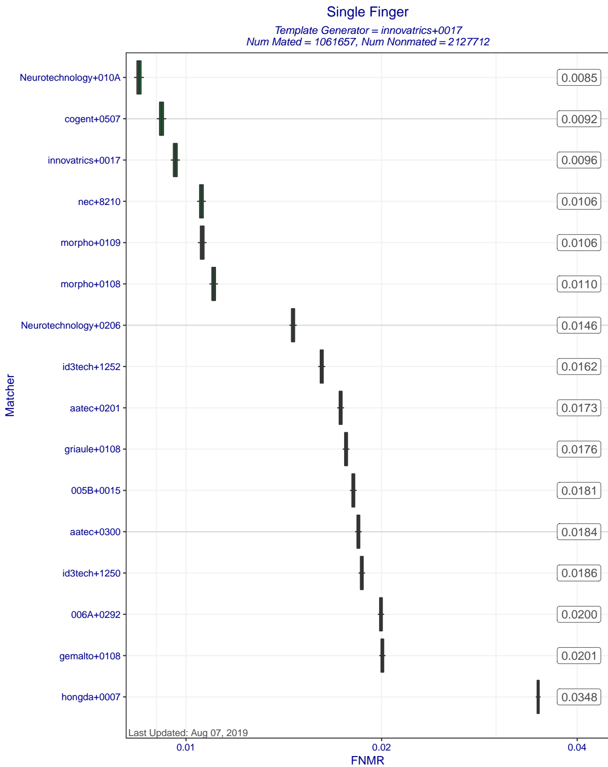
Figure 5: Single Finger FNMRs at FMR=0.0001 when MINEX III compliant matchers compare templates created by template generator innovatrics+0017. Each box represents uncertainty about the true FNMR. The box edges mark the 50% confidence intervals while the whiskers mark the 90% confidence intervals. The numbers on the right show the actual computed FNMRs.
