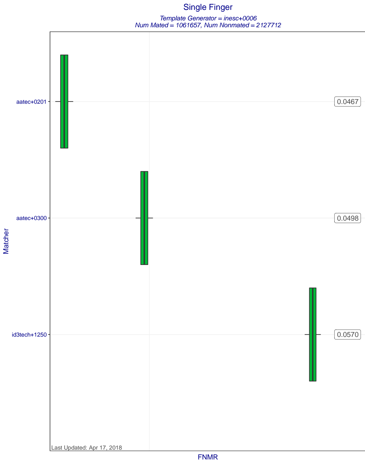
Figure 5: Single Finger FNMRs at FMR=0.0001 when MINEX III compliant matchers compare templates created by template generator inesc+0006. Each box represents uncertainty about the true FNMR. The box edges mark the 50% confidence intervals while the whiskers mark the 90% confidence intervals. The numbers on the right show the actual computed FNMRs.
