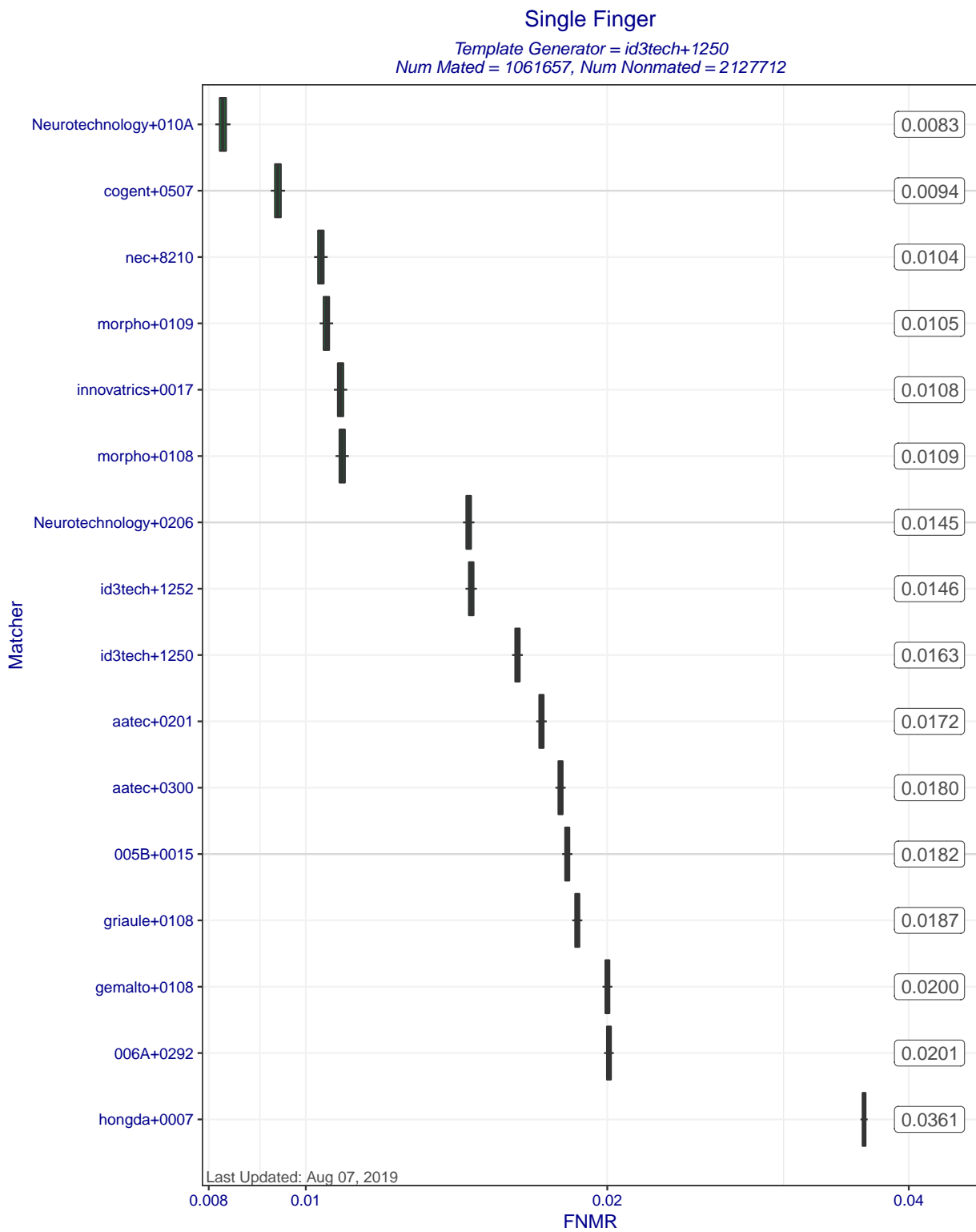
Figure 5: Single Finger FNMRs at FMR=0.0001 when MINEX III compliant matchers compare templates created by template generator id3tech+1250. Each box represents uncertainty about the true FNMR. The box edges mark the 50% confidence intervals while the whiskers mark the 90% confidence intervals. The numbers on the right show the actual computed FNMRs.
