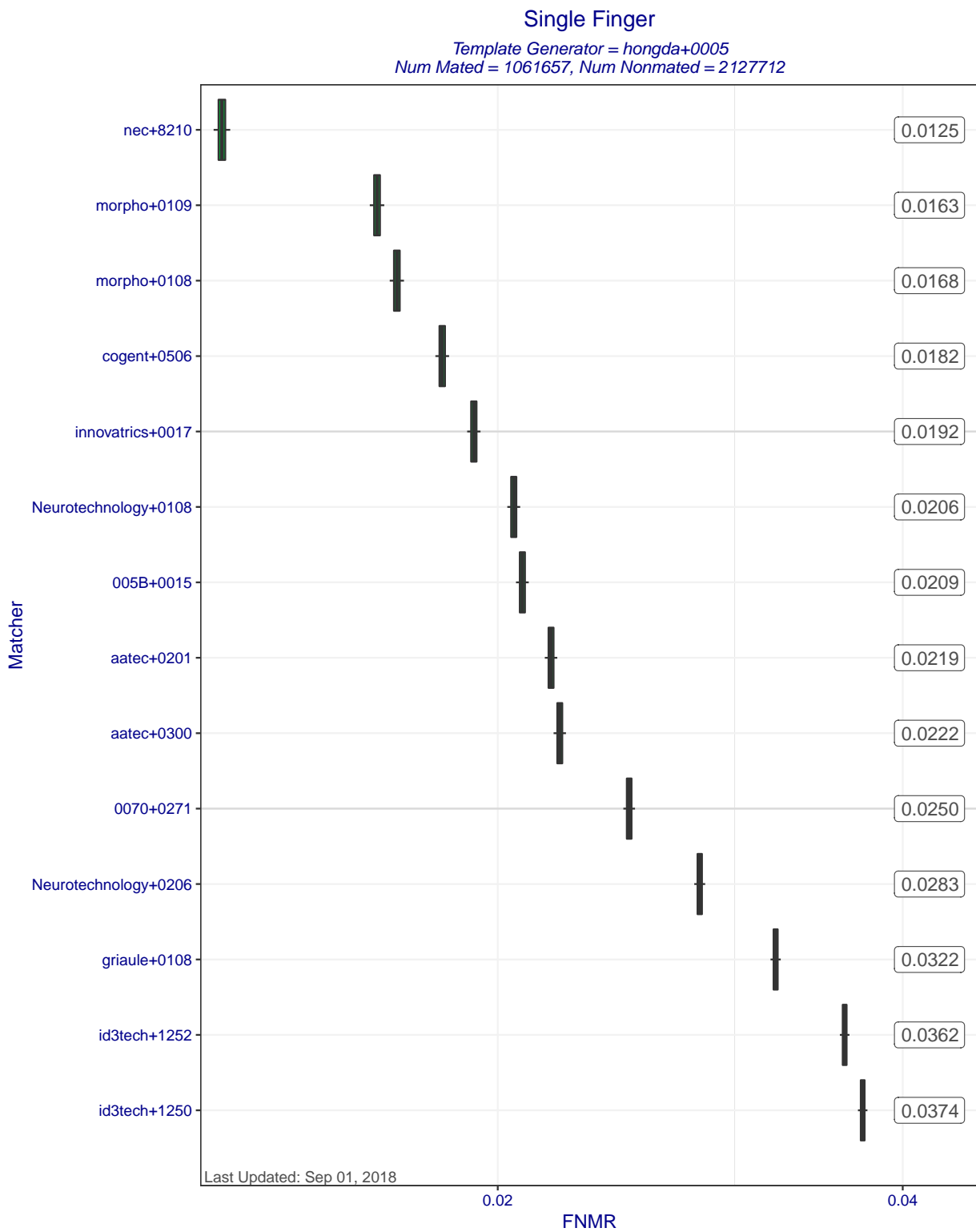
Figure 5: Single Finger FNMRs at FMR=0.0001 when MINEX III compliant matchers compare templates created by template generator hongda+0005. Each box represents uncertainty about the true FNMR. The box edges mark the 50% confidence intervals while the whiskers mark the 90% confidence intervals. The numbers on the right show the actual computed FNMRs.
