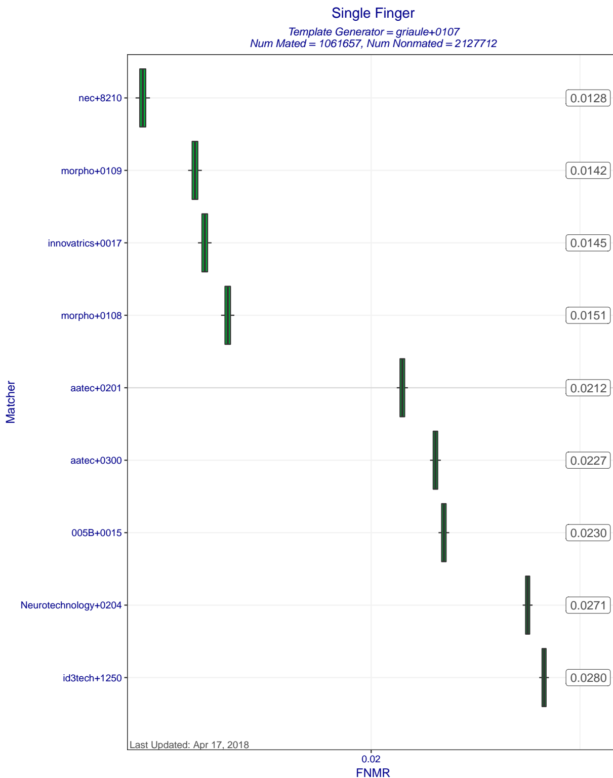
Figure 5: Single Finger FNMRs at FMR=0.0001 when MINEX III compliant matchers compare templates created by template generator griaule+0107. Each box represents uncertainty about the true FNMR. The box edges mark the 50% confidence intervals while the whiskers mark the 90% confidence intervals. The numbers on the right show the actual computed FNMRs.
