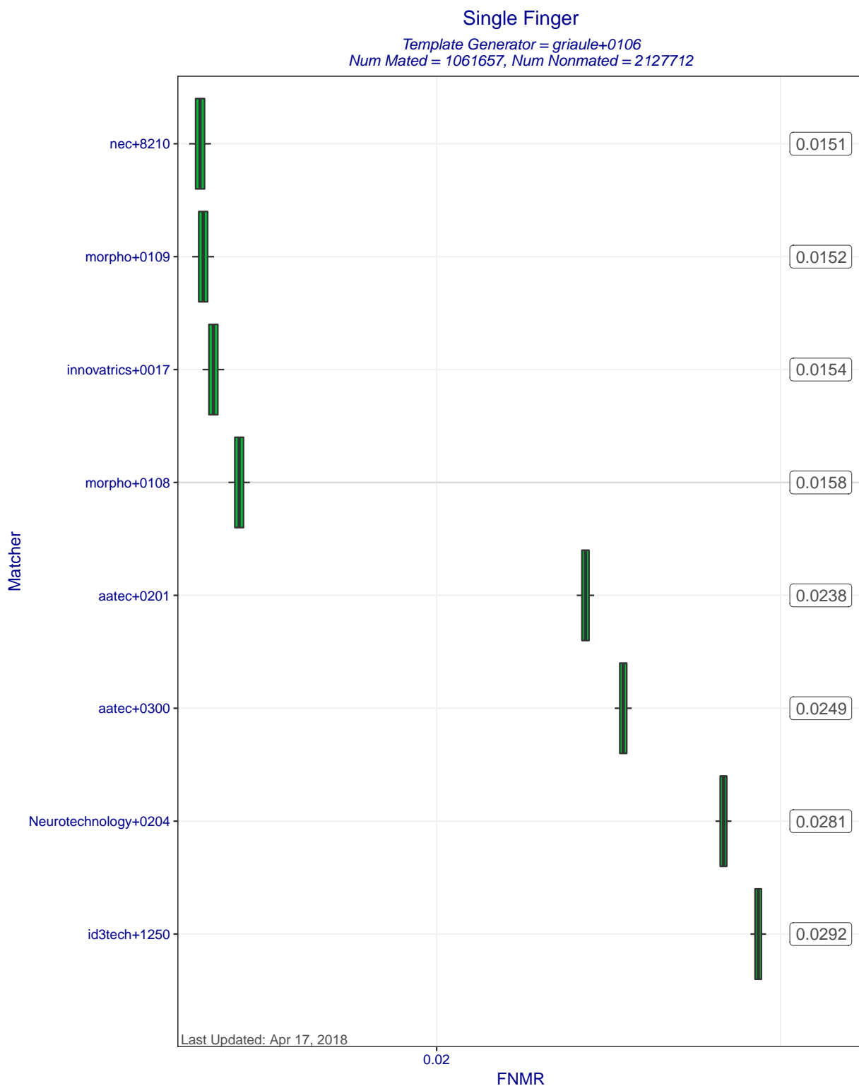
Figure 5: Single Finger FNMRs at FMR=0.0001 when MINEX III compliant matchers compare templates created by template generator griaule+0106. Each box represents uncertainty about the true FNMR. The box edges mark the 50% confidence intervals while the whiskers mark the 90% confidence intervals. The numbers on the right show the actual computed FNMRs.
