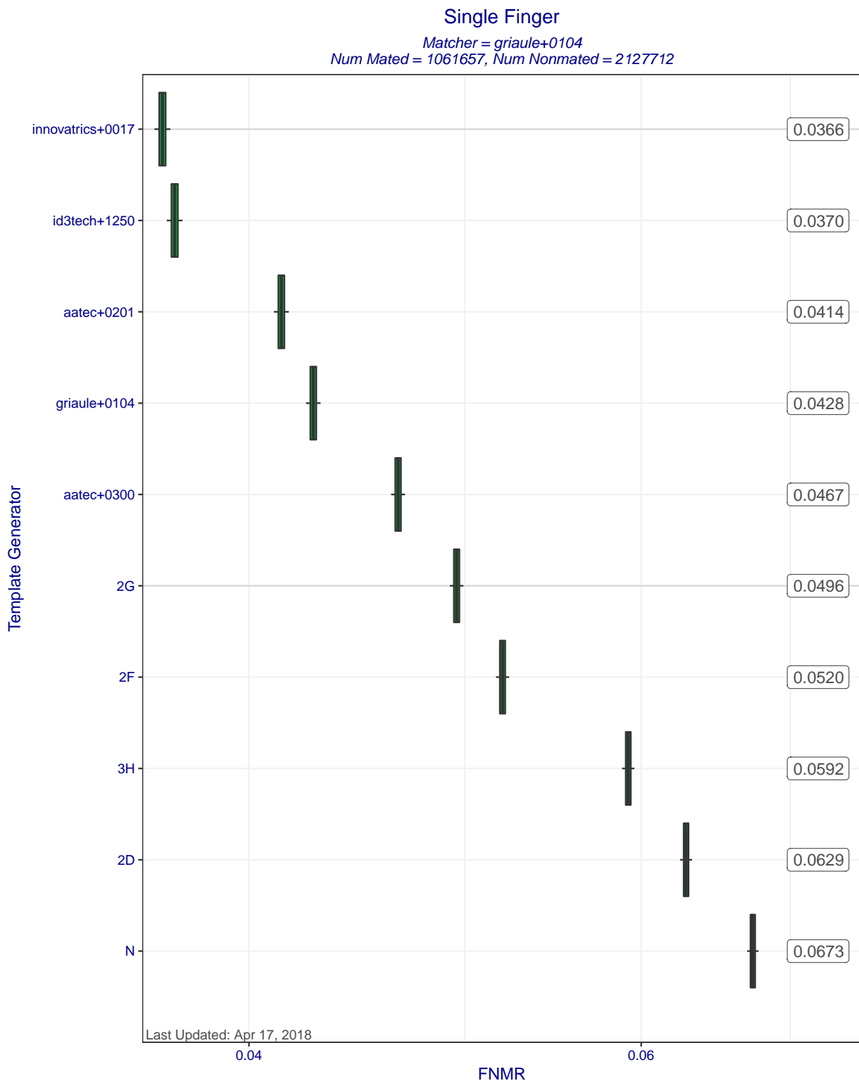
Figure 5: Single finger FNMRs at FMR = 0.0001 when matcher griaule+0104 compares templates created by different template generators. The ends of the whiskers show the minimum and maximum FNMRs. Each box represents uncertainty about the true FNMR. The box edges mark the 50% confidence intervals while the whiskers mark the 90% confidence intervals. The numbers on the right show the actual computed FNMRs.
