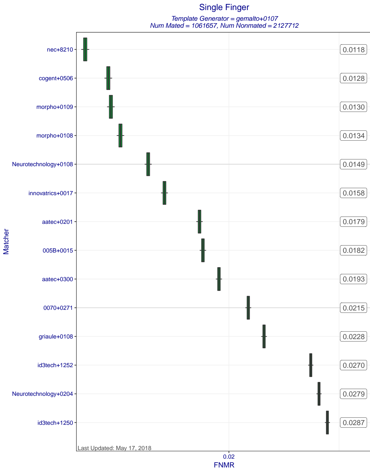
Figure 5: Single Finger FNMRs at FMR=0.0001 when MINEX III compliant matchers compare templates created by template generator gemalto+0107. Each box represents uncertainty about the true FNMR. The box edges mark the 50% confidence intervals while the whiskers mark the 90% confidence intervals. The numbers on the right show the actual computed FNMRs.
