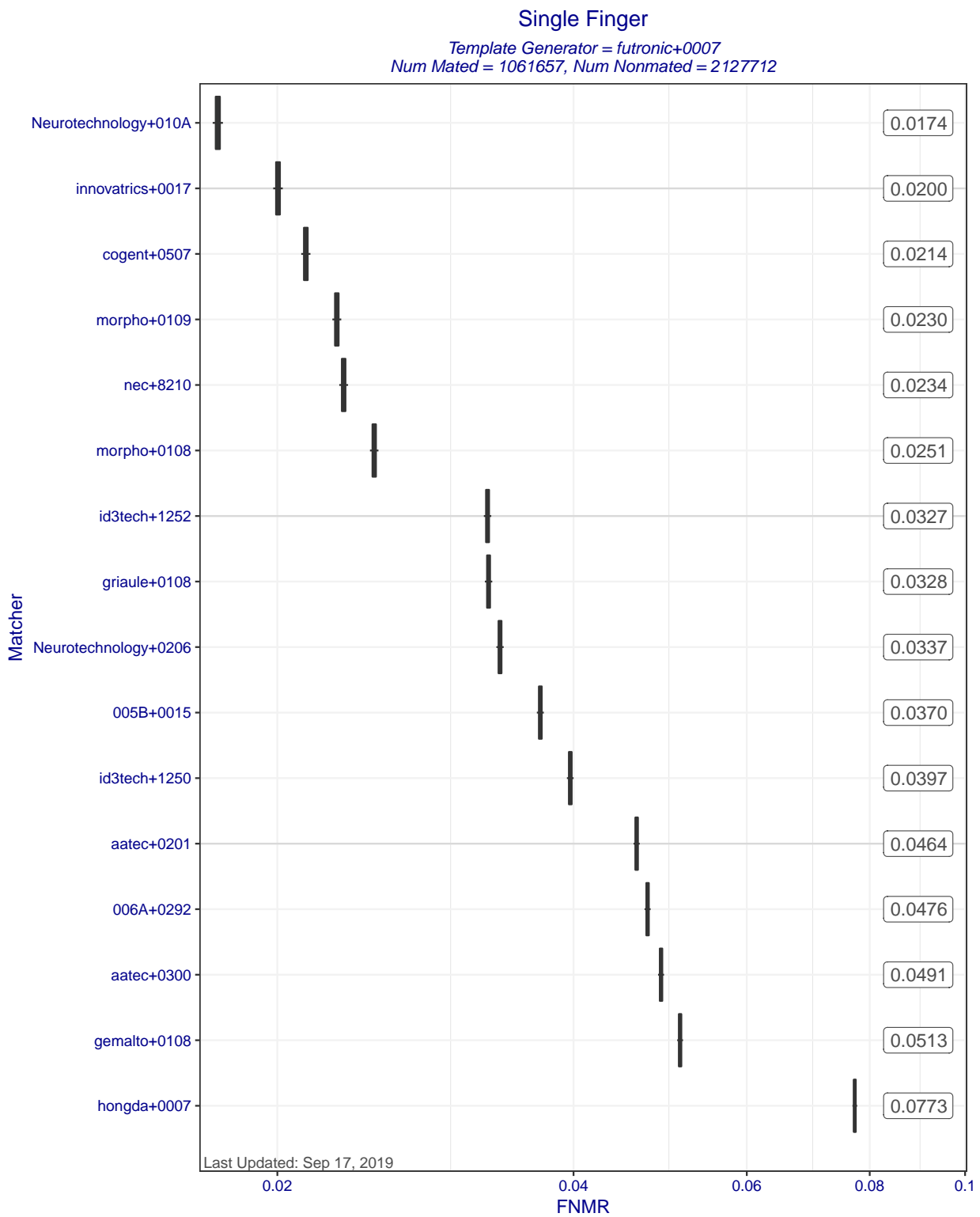
Figure 5: Single Finger FNMRs at FMR=0.0001 when MINEX III compliant matchers compare templates created by template generator futronic+0007. Each box represents uncertainty about the true FNMR. The box edges mark the 50% confidence intervals while the whiskers mark the 90% confidence intervals. The numbers on the right show the actual computed FNMRs.
