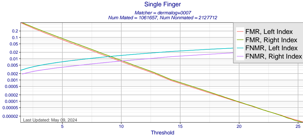
Figure 11: Single finger FMR and FNMR as a function of score threshold for matcher dermalog+0007 using templates created by all MINEX III compliant template generators. Separate curves are presented for left and right index fingers.
