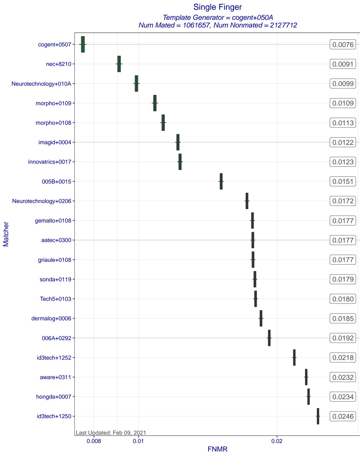
Figure 5: Single Finger FNMRs at FMR=0.0001 when MINEX III compliant matchers compare templates created by template generator cogent+050A. Each box represents uncertainty about the true FNMR. The box edges mark the 50% confidence intervals while the whiskers mark the 90% confidence intervals. The numbers on the right show the actual computed FNMRs.
