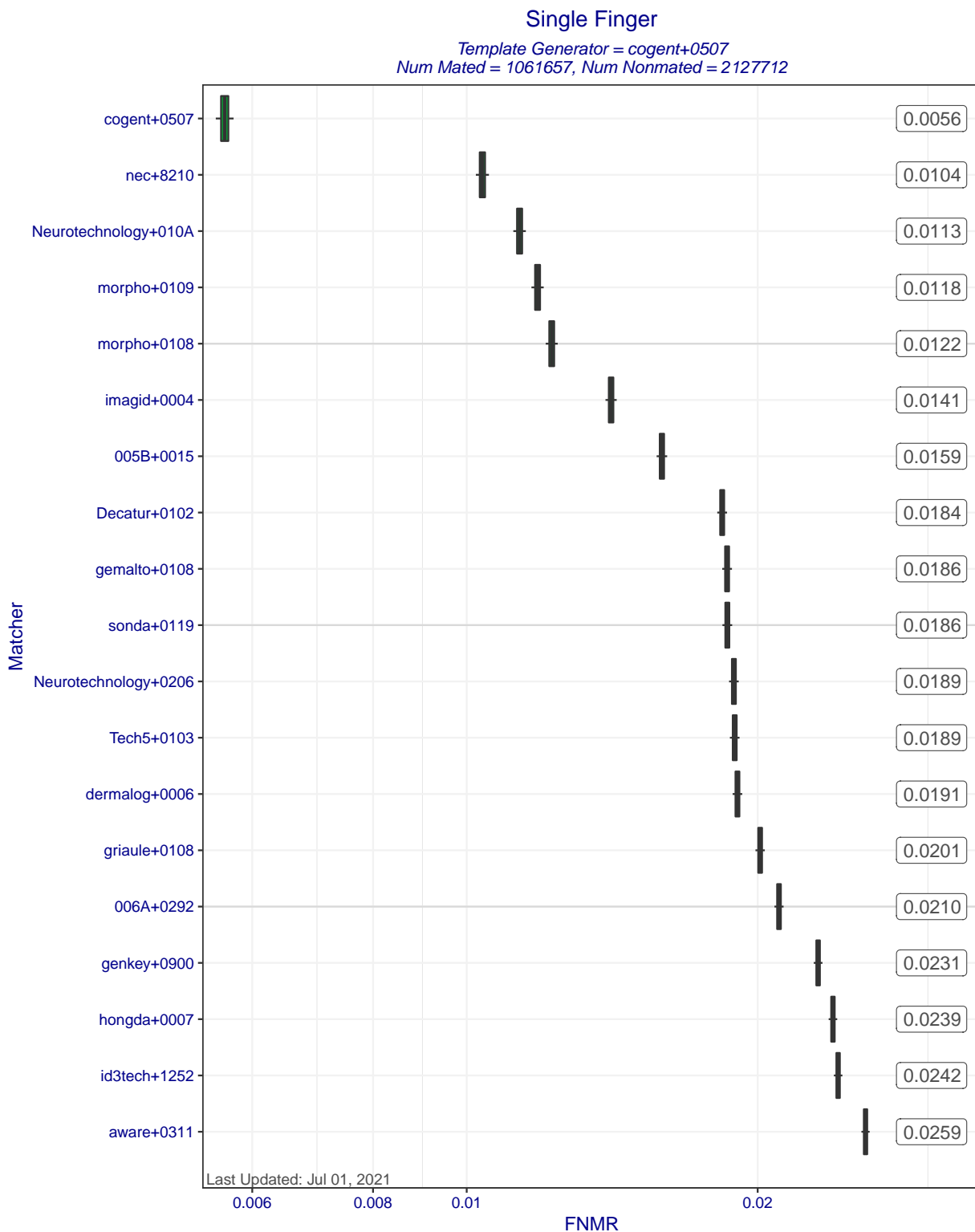
Figure 5: Single Finger FNMRs at FMR=0.0001 when MINEX III compliant matchers compare templates created by template generator cogent+0507. Each box represents uncertainty about the true FNMR. The box edges mark the 50% confidence intervals while the whiskers mark the 90% confidence intervals. The numbers on the right show the actual computed FNMRs.
