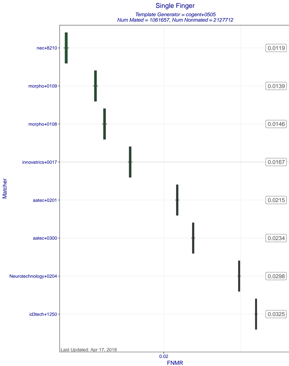
Figure 5: Single Finger FNMRs at FMR=0.0001 when MINEX III compliant matchers compare templates created by template generator cogent+0505. Each box represents uncertainty about the true FNMR. The box edges mark the 50% confidence intervals while the whiskers mark the 90% confidence intervals. The numbers on the right show the actual computed FNMRs.
